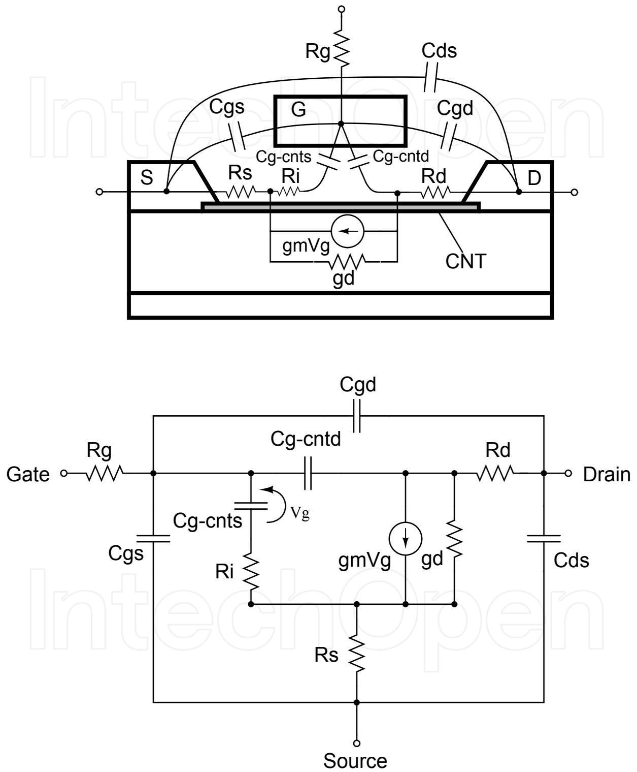
Fig. 7. Equivalent small-signal circuit model for CNTFET.
