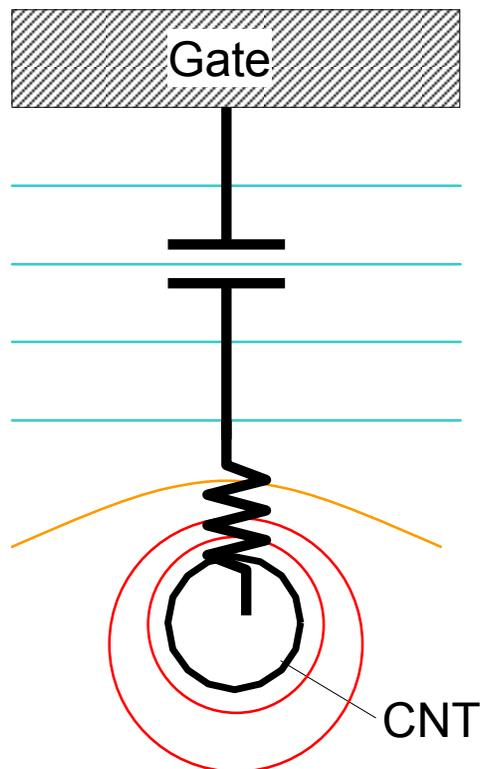
Fig. 10. Equivalent circuit between gate electrode and CNT
