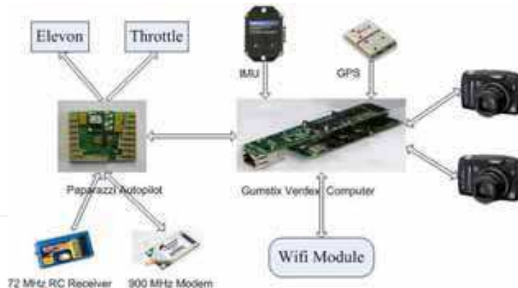
Fig. 8. AggieAir Airborne System Structure.
