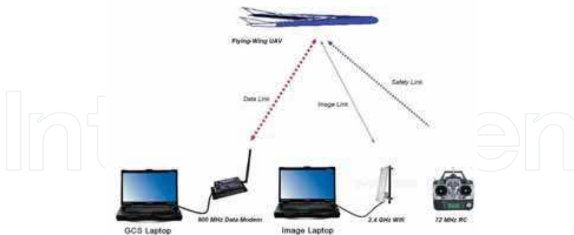
Fig. 6. AggieAir UAS Physical Structure.
