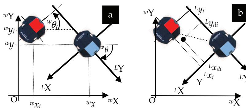
Figure 1. a) Reference systems: world (absolute) reference coordinate system ( $O wX wY$ ), and a second coordinate system attached to the leader robot ( $O LX LY$ ) where the desired positions for each of the followers are defined. b)  $i$ -th follower robot positioned at coordinates  $({}^L x_i, {}^L y_i)$  on the leader Cartesian reference where the reference position is given by  $({}^L x_{di}, {}^L y_{di})$
