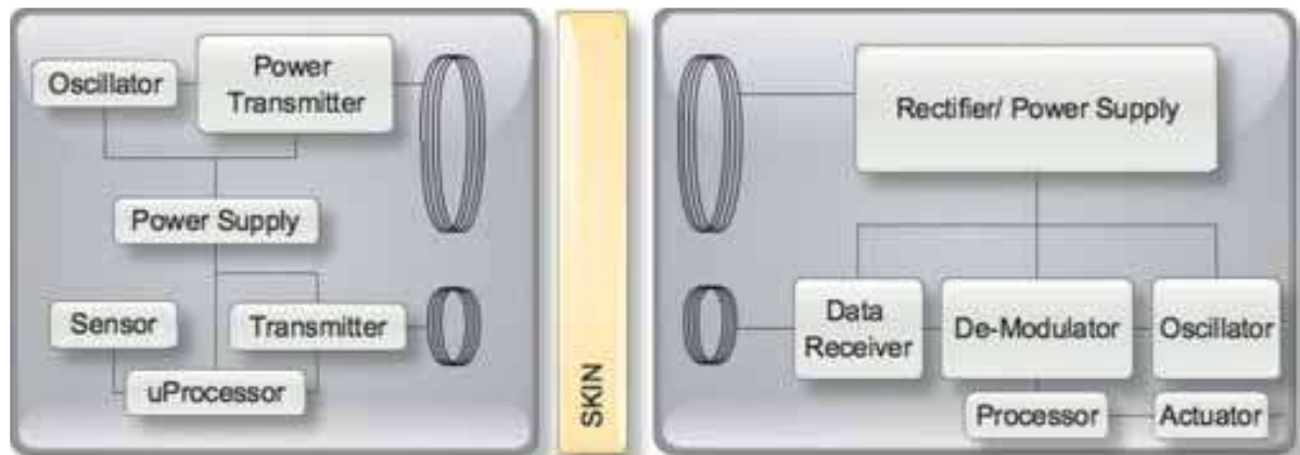
Fig. 2. A block diagram of a prosthesis system, where the external element is on the left and the internal element on the right.
