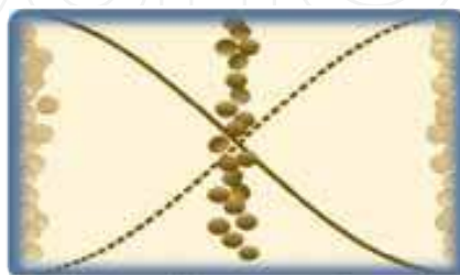
Fig. 3. Generation of an ultrasonic standing wave in a channel which length equals \lambda/2 . Particles having a positive acoustic contrast factor ( \phi > 0 ) are directed to the chamber midplane toward the pressure node, whereas particles having \phi < 0 collect at the chamber walls (pressure anti-nodes).
