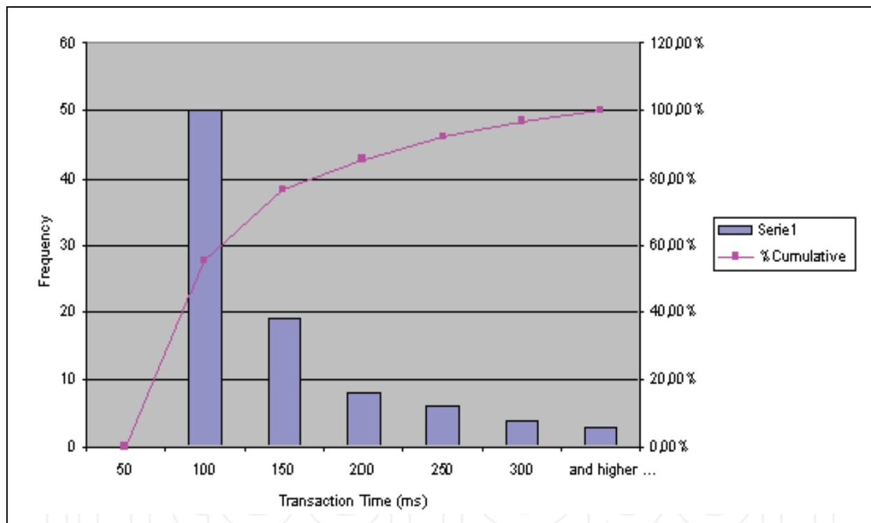
Fig. 12. Histogram with transaction times for Bluetooth technology.
