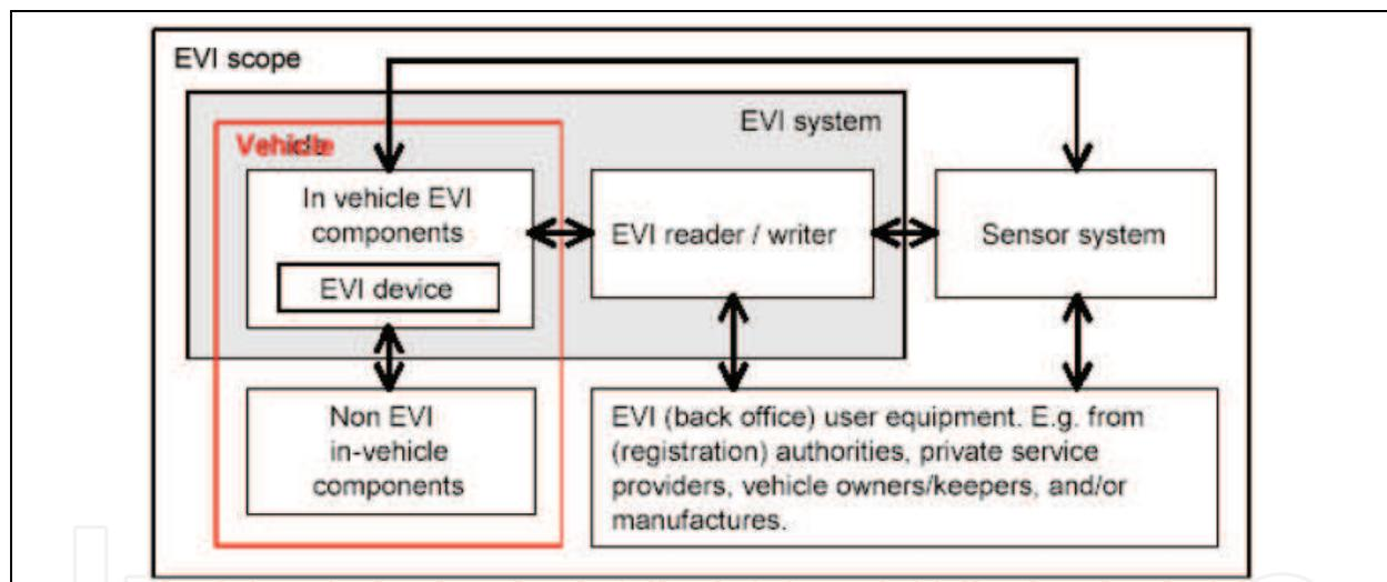
Fig. 2. Schema of components in the EVI scope
