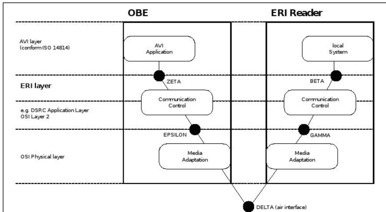
Fig. 1. ERI within the AVI/AEI reference architecture framework.
