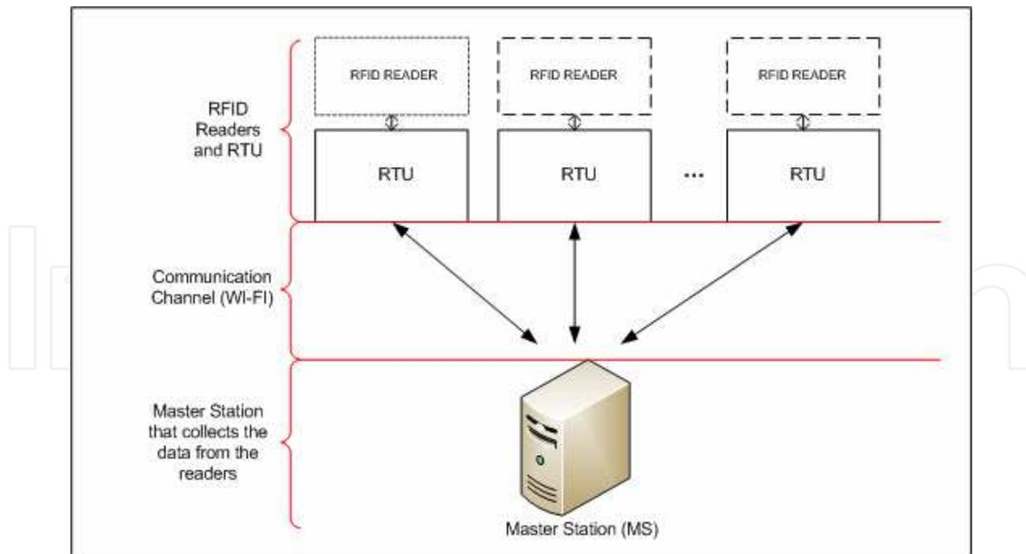
Fig. 14. A Minimal SCADA system (IEEE, 1994).
