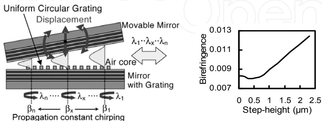
Fig. 13. (a) Schematic of tapered 3D hollow waveguide Bragg reflector (b) calculated birefringence (of straight hollow waveguide) versus step height  $h$  at an air core thickness  $D = 5 \mu\text{m}$  and step width  $W = 10 \mu\text{m}$ .
