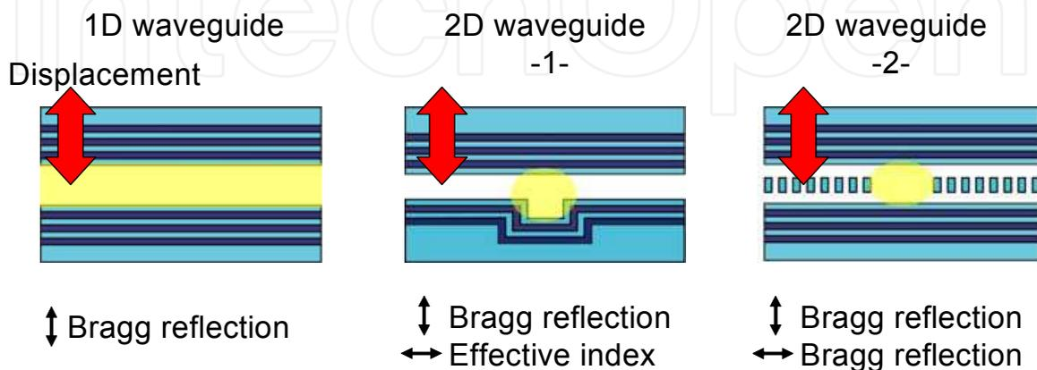
Fig. 3. Tunable Hollow optical waveguide structures [38]-[40].
