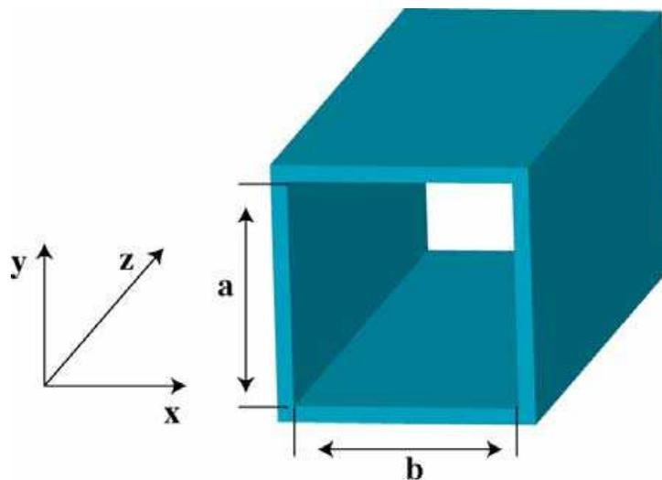
Fig. 4. Assumed 3D hollow waveguide model for analysis.
