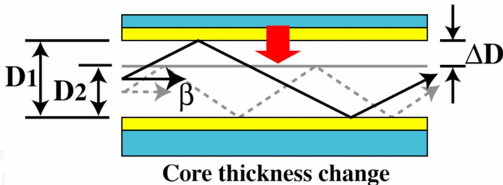
Fig. 6. Conceptual diagram of propagation constant tuning.
