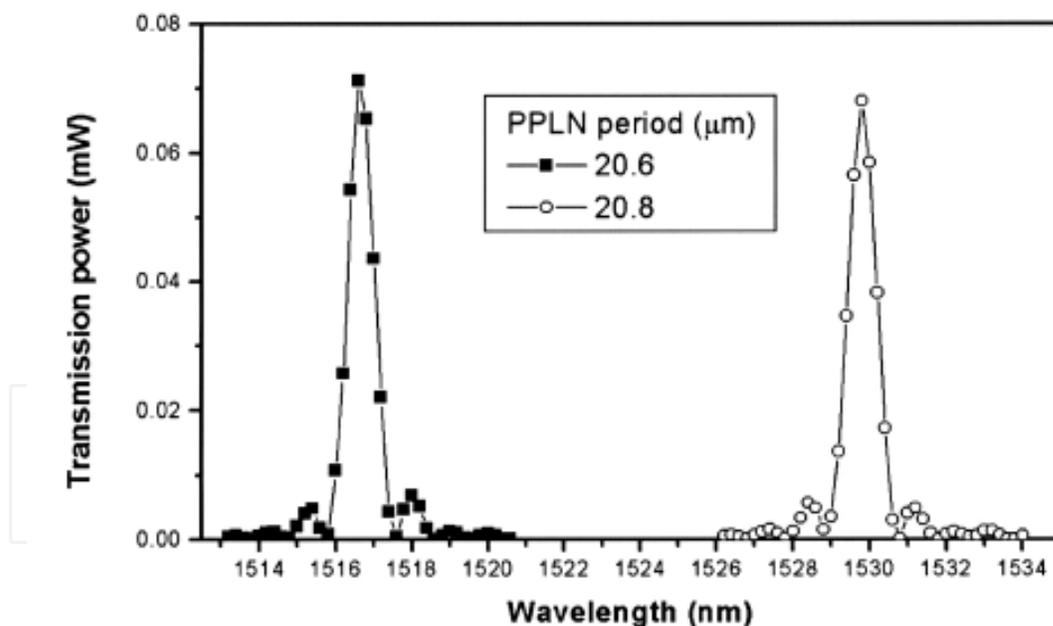
Fig. 3. Measured transmission power versus wavelength of the Solc filter in the 20.6- and 20.8-mm-period PPLN at a temperature of 24 °C. The FWHM of the transmission spectrum is  $\sim 0.8$  nm(Chen et al.,2003).
