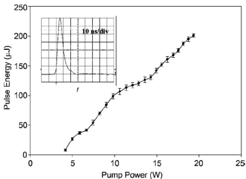
Fig. 28. Output pulse energy of the actively Q-switched Nd:YVO<sub>4</sub> laser versus pump power. With 19.35 W pump power at 808 nm, the 1064 nm laser pulse has an energy of 201  $\mu$ J and a width of 7.8 ns, corresponding to a laser peak power of 26 kW. The inset shows the measured temporal profile of the Q-switched laser pulse (Y.Y.Lin et al.,2007).
