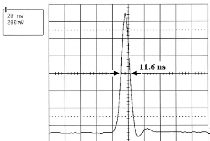
Fig. 26. Measured Q-switched pulse from the EO PPLN Q-switched Nd:YVO<sub>4</sub> laser at 1.2-W pump power. The pulse width was 11.6 ns, and the peak power was  $\sim 0.74$  kW(Chen & Huang,2003).
