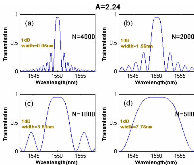
Fig. 10. The transmission spectrums by use of numeral calculation in PPLN with the product  $A$  fixed at 2.24. (a) The transmission spectrum with  $N$  at 4000; (b) The transmission spectrum with  $N$  at 2000; (c) The transmission spectrum with  $N$  at 1000; (d) The transmission spectrum with  $N$  at 500(Liu et al.,2009a).
