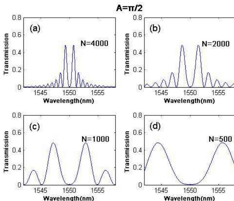
Fig. 9. The transmission spectrums by use of numeral calculation in PPLN with the product  $A$  fixed at  $\pi/2$ . (a) The transmission spectrum with  $N$  at 4000; (b) The transmission spectrum with  $N$  at 2000; (c) The transmission spectrum with  $N$  at 1000; (d) The transmission spectrum with  $N$  at 500(Liu et al.,2009a).
