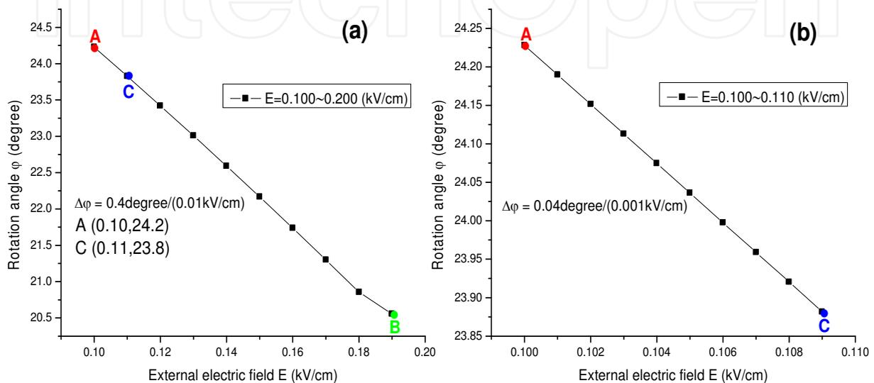
Fig. 21. Experimental measurement of the rotation angle of the output light ( $\lambda=1543.47\text{nm}$ ) when varying the applied electric field with smaller step. (a) The external electric field varies from 0.100 to 0.200 (kV/cm); (b) The external electric field varies from 0.100 to 0.110 (kV/cm) (Liu et al.,2009c).
