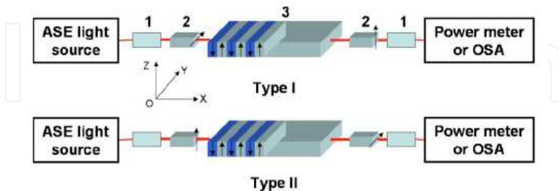
Fig. 13. Two types of device setups for PPLN Solc-type wavelength filter; the arrow on the polarizer indicates the polarization direction. The fact that type A takes on the filter behavior while type B does not reveals the test light has the PVE on the PPLN and it becomes a Solc filter when no external field exists. The numbered components are: 1, collimator; 2, crossed polarizer; 3, PPLN(Chen et al.,2006).
