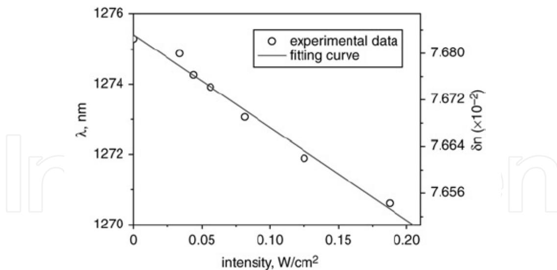
Fig. 18. Centre wavelength of Ti:PPLN solc-type filter against UV illumination intensity (Lee et al., 2008)
