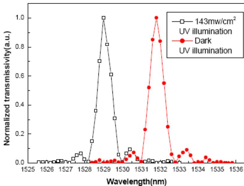
Fig. 15. The spectrum of the PPLN filter under  $143\text{mW}/\text{cm}^2$  UV illumination (empty square symbol) and without UV light illumination (red circle symbol) (Shi et al.,2006).
