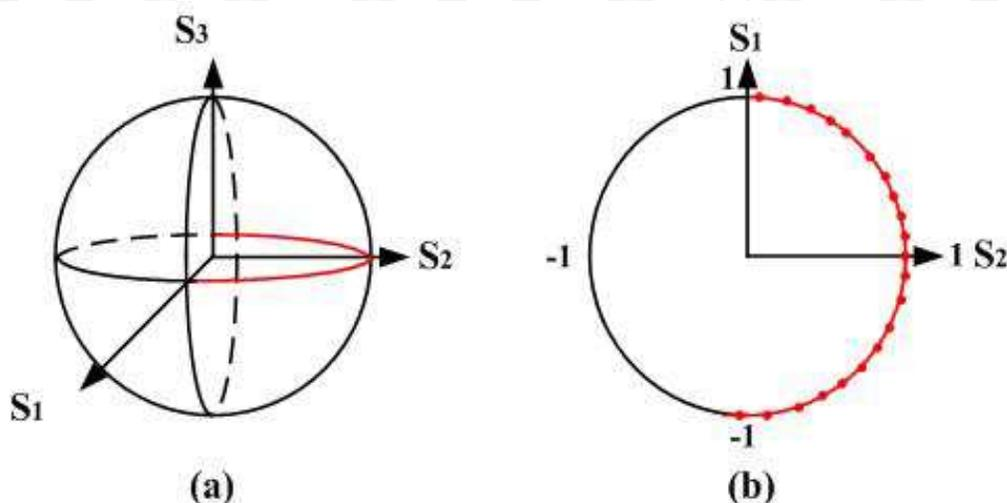
Fig. 19. Experimental measurement of the state of polarization of the output light ( $\lambda=1543.47\text{nm}$ ) on a Poincare sphere when varying the applied electric field from 0 to 3 (kV/cm) (Liu et al.,2009c).
