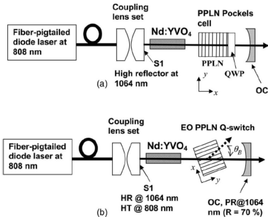
Fig. 27. Schematic of the actively Q-switched Nd:YVO<sub>4</sub> laser using (a) a PPLN Pockels cell and (b) an EO PPLN Bragg modulator as a laser Q-switch. The laser cavity is formed by the surface S1 and the output coupler (OC). In (b), the Bragg angle  $\theta_B$  is exaggerated for clarity. QWP, quarter-wave plate; HR, high reflection; HT, high transmission; PR, partial reflection (Y.Y.Lin et al,2007).
