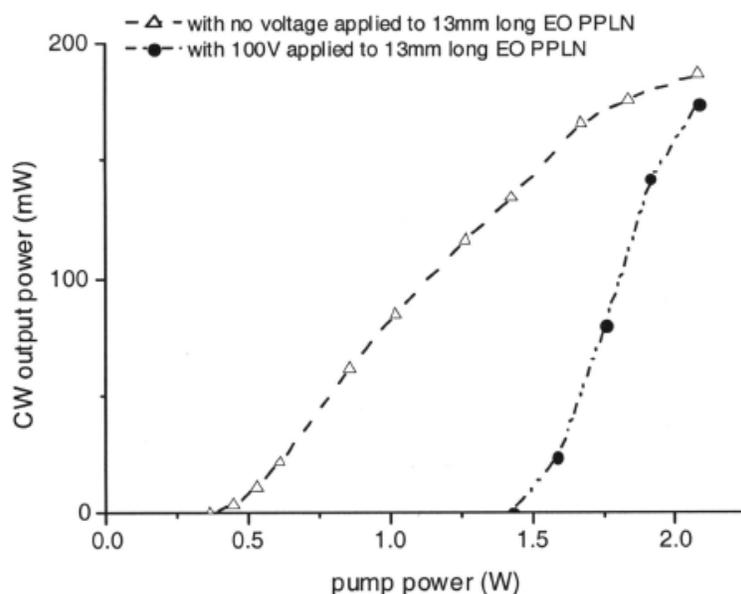
Fig. 25. CW performance of the Nd:YVO<sub>4</sub> laser with (solid curve) and without (dashed curve) a 100-V voltage applied to the EO PPLN. With the 100-V voltage, the laser threshold was increased from 400 mW to 1.4 W because of the polarization-rotation effect from the EO PPLN crystal(Chen & Huang,2003).
