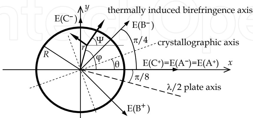
Fig. 2. Cross-section of magneto-optical crystal:  $r$ ,  $\varphi$  are polar coordinates;  $\theta$  is angle of inclination of the crystallographic axis;  $\Psi$  is angle of inclination of eigen polarization of thermally induced birefringence.
