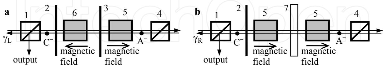
Fig. 9. FI designs with a  $\lambda/2$  plate (a) and QR (b) (Khazanov, 1999). 1,4 - polarizers, 2,3 -  $\lambda/2$  plates, 5 -  $22.5^\circ$  MOE rotating clockwise, 6 -  $22.5^\circ$  MOE rotating anticlockwise, 7 -  $67.5^\circ$  QR.
