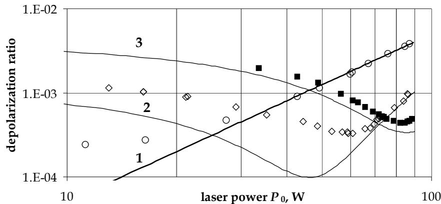
Fig. 8. Depolarization ratio in traditional FI design  $\gamma(P_0)$  (curve 1, circles) and design in Fig. 7  $\gamma_q(P_0)$  at  $f=125\text{mm}$  (curve 2, rhombs) and  $f=88\text{mm}$  (curve 3, squares) (Andreev et al., 2002).
