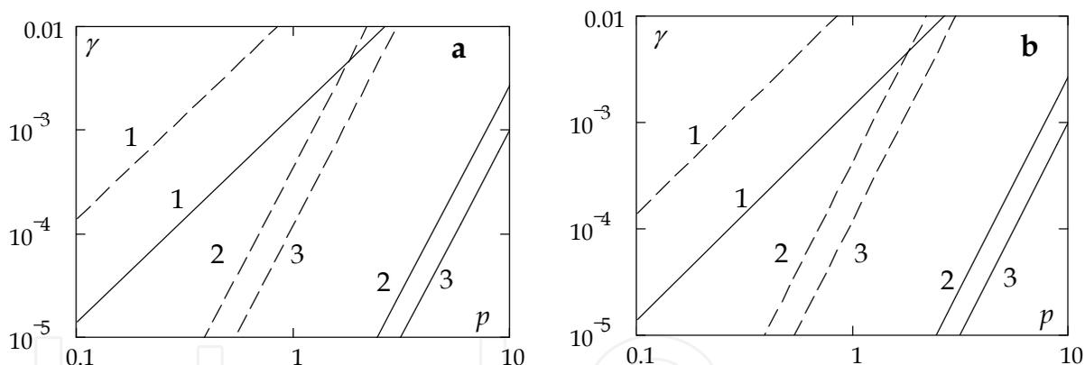
Fig. 17. The plots (solid lines) of  $\gamma_{slab}(p)$  for TGG-based FI with slab,  $R_s=4$  (a) and  $\gamma_{disc}(p)$  for glass-based FI with discs,  $R_d=1.8$  (b). 1 - FI design in Fig. 1; 2 - FI design in Fig. 9a; 3 - FI design in Fig 9b. Dashed lines show  $\gamma$  as a function of  $p$  for rods.
