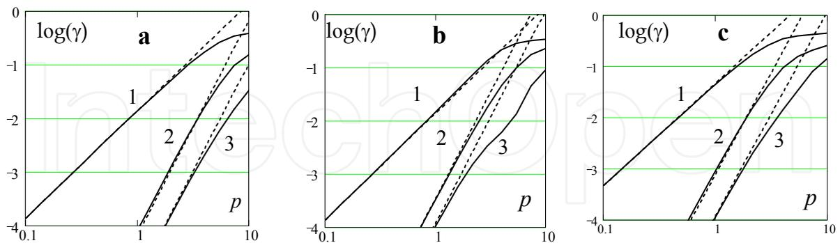
Fig. 10. Numerical (solid curves) and analytical (22, 36, 38) (dashed) plots of  $\gamma(p)$  for the traditional FI design in Fig. 1 (1),  $\gamma_L(p)$  for FI design with a  $\lambda/2$  plate in Fig. 9a (2), and  $\gamma_R(p)$  for FI design with QR in Fig 9b (3). (a) glass (b) TGG crystal with the [001] orientation, and (c) TGG crystal with the [111] orientation.
