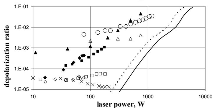
Fig. 11. Experimental plots of  $\gamma(P_0)$  (filled symbol) and  $\gamma_R(P_0)$  (open symbol) for different FIs: (Andreev et al., 2000b) (rhombs), (Nicklaus et al., 2006) (circles), (Voytovich et al., 2007) (squares, triangles), and unpublished data (crosses). Theoretical curves correspond to  $\gamma_R(P_0)$  for squares (solid) and triangles (dashed).
