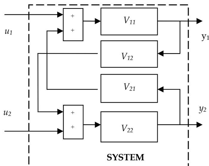
Fig. 6. The exemplary V-structure for 2 inputs and 2 outputs.
