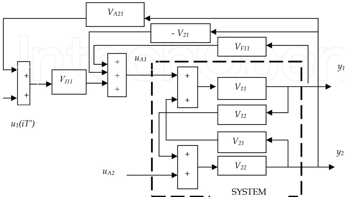
Fig. 7. The synthesis of signal  $u_{A1}$  for scaling of SYSTEM output signal  $y_1$ . To avoid the illegibility of scheme the sub-structure generating signal  $u_{A2}$  has not been attached. Note, that effect of time-scaling has been achieved without modification of internal structure of SYSTEM.
