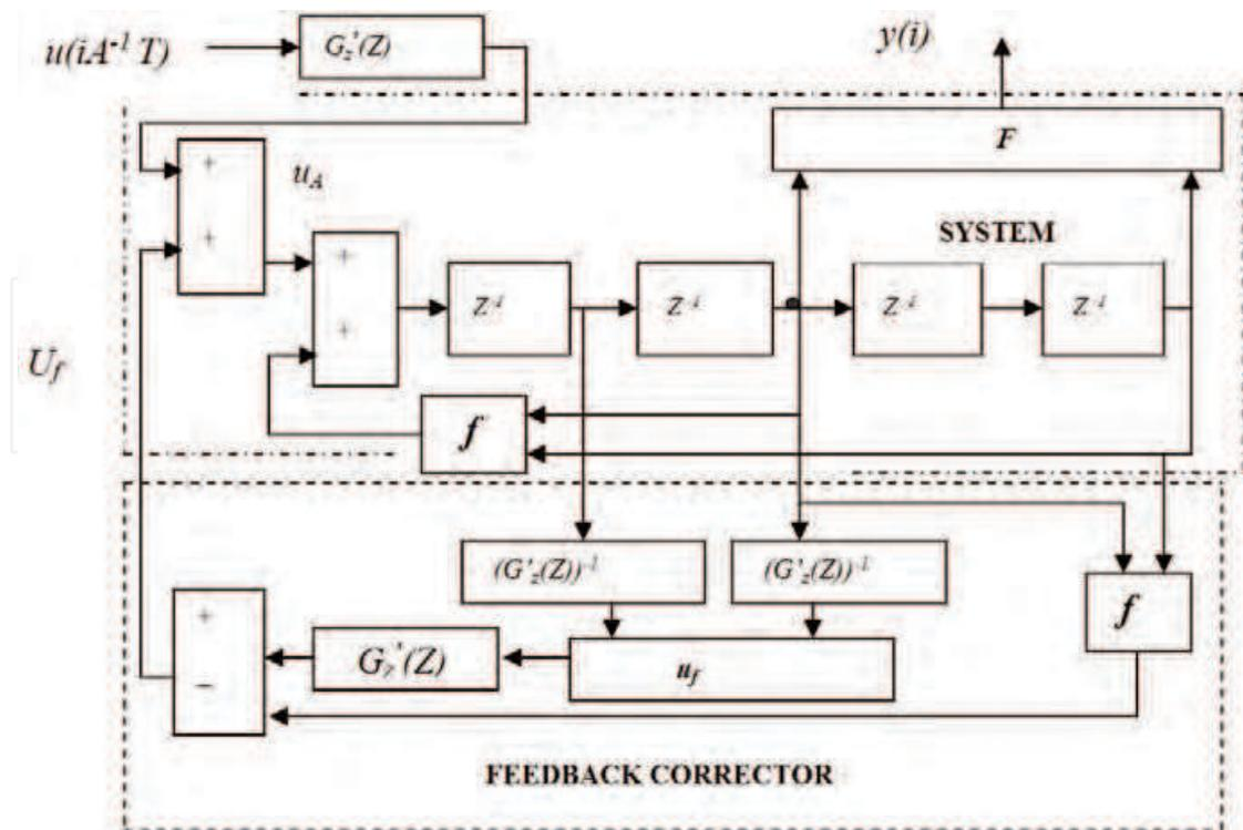
Fig. 4. The scaling of system (6) according to Fig. 2 and matter of *Example B*. Note, that primary delays  $T$  (for  $z^{-1}$ ) are substituted with the two delays  $T' = 0.5 T$ , where  $T'$  refers to operator  $Z^{-1}$ .
