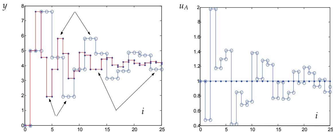
Fig. 3. **Left position:** the reference response of system (6) to signal  $u(i) = 1(i)$  – curve distinguished by "." – and response of system (6) obtained as output signal of structure in Fig. 2 – curve distinguished by "o". Note, that consecutive amplitudes of both responses are identical (compare chosen referring amplitudes indicated by arrows). **Right position:** reference input signal  $u(i) = 1(i)$  and input signal  $u_A(i)$  of system (6) when included to structure in Fig. 2 as SYSTEM.
