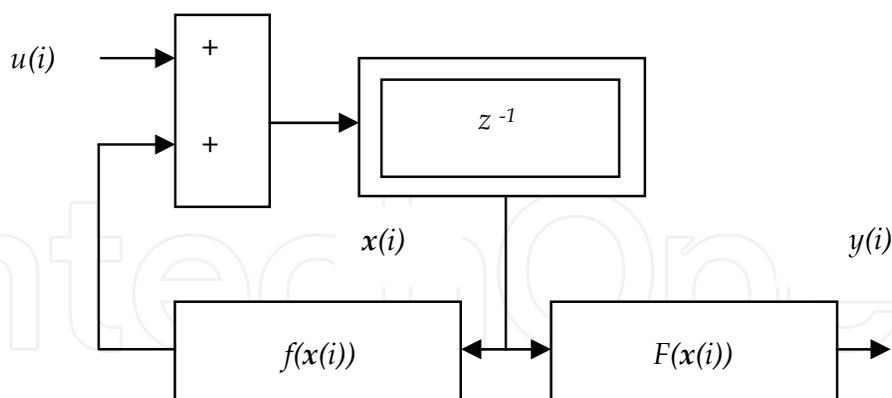
Fig. 1. The simplified scheme of system (1):  $z^{-1}$  - chain of unit delay elements,  $x(i)$  -state vector with components representing outputs of single delay elements,  $F$  and  $f$  - static nonlinear functions,  $u$  -input,  $y$  - output.
