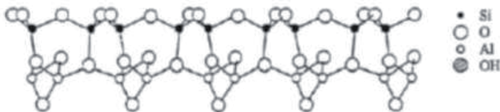
Figure 1. Structure of kaolinite designed by Brindley and Nakahira viewed from the a-axis direction [23].
