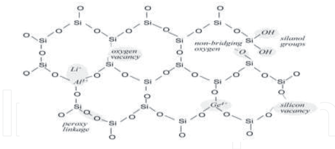
Figure 2. Schematic structure of quartz [27].
