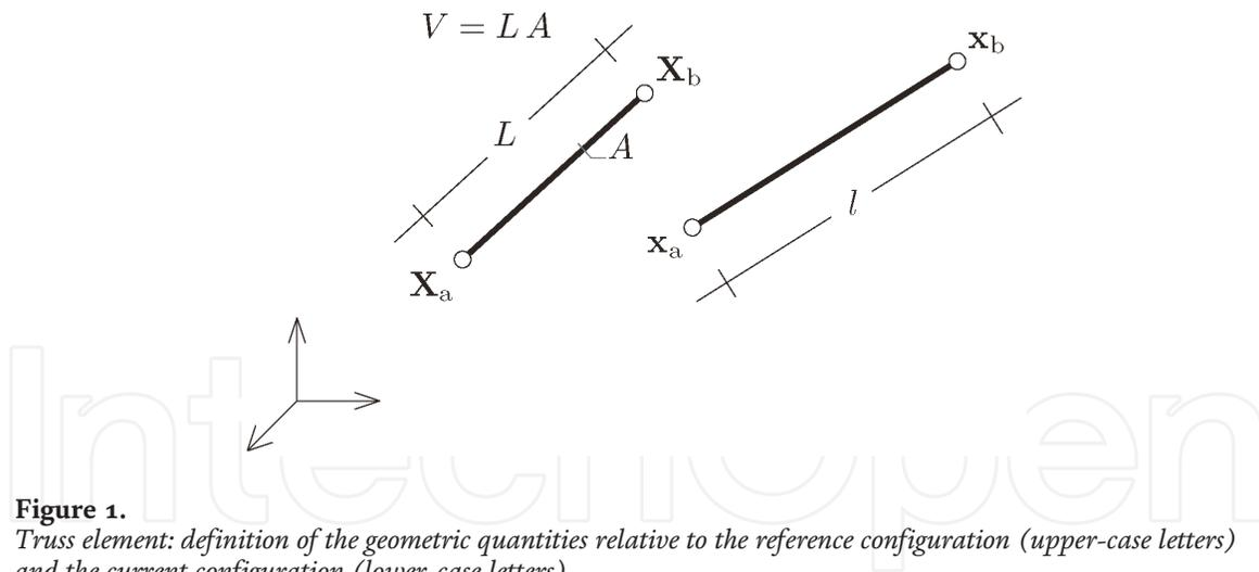
**Figure 1.** Truss element: definition of the geometric quantities relative to the reference configuration (upper-case letters) and the current configuration (lower-case letters).
