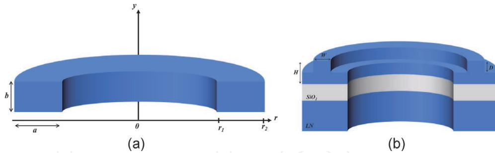
**Figure 2.** (a) Toroidal waveguide with a width of core,  $a = r_2 - r_1 = 1 \mu\text{m}$  and height,  $b = 0.5 \mu\text{m}$  where  $r_1 = 0.5 \mu\text{m}$  and  $r_2 = 1.5 \mu\text{m}$ . (b) LNOI rib waveguide with the thickness of the slab,  $h = H - D$  [17].
