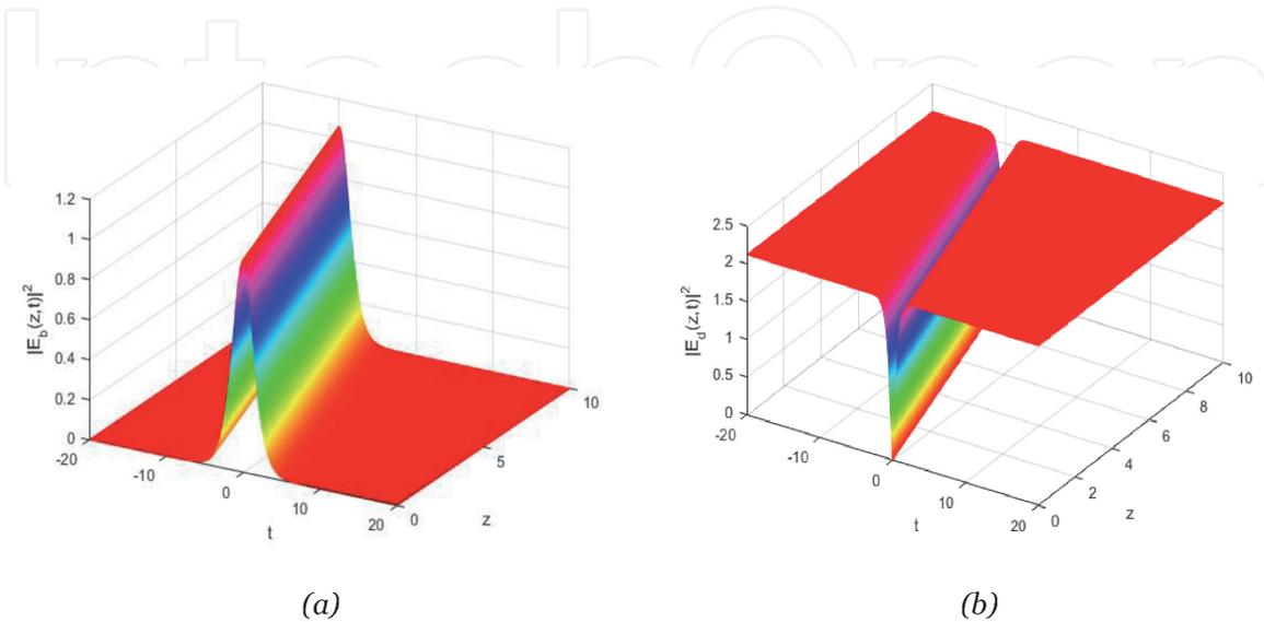
**Figure 1.** Intensity  $|E_j(z, t)|^2$  distribution of the (a) bright and (b) dark solitons given by Eqs. (14) and (17), respectively, with the parameter values corresponding to CQNLS models as  $\alpha_1 = 0.5$ ,  $\alpha_2 = 0$ ,  $\alpha_3 = 1$ ,  $\alpha_4 = 0$ ,  $\alpha_5 = 0$ ,  $k = 1$ , and  $\omega = 1$ .
