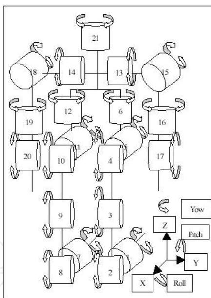
Fig. 2. The movable range of the servomotors.
