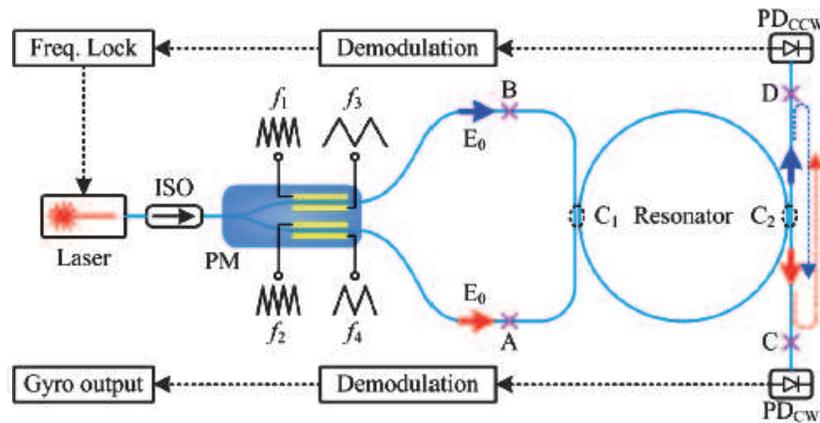
**Figure 7.** Conventional configuration of an IORG, including a narrow linewidth laser source, an optical isolator, optoelectronic components for demodulation processing, a waveguide ring resonator, two detectors, and electronics readout unit.
