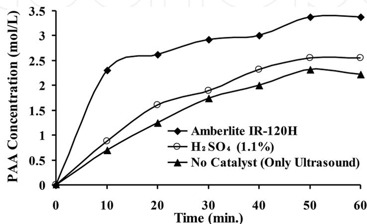
**Figure 8.** Comparative study on the activity of different catalyst during PAA formation (molar ratio of acetic acid to  $\text{H}_2\text{O}_2 = 1:1$ , catalyst loading of Amberlite IR-120H =  $471 \text{ mg/cm}^3$ , temperature =  $40^\circ\text{C}$ ).
