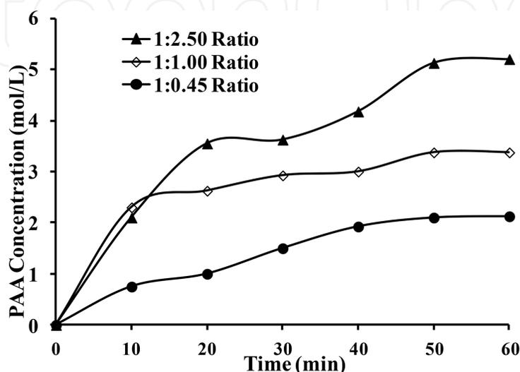
**Figure 2.** Effect of molar ratio of acetic acid to hydrogen peroxide on PAA formation (catalyst loading = 471 mg/cm<sup>3</sup>, temperature = 40°C) in batch reactor.
