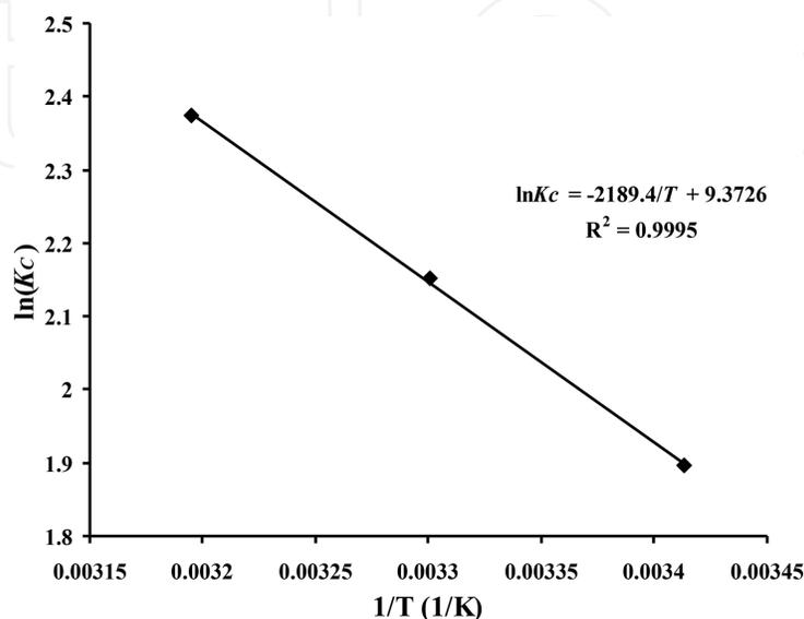
**Figure 5.** The Arrhenius plot of equilibrium constant at different temperature (in kelvin) for PAA formation (molar ratio of acetic acid to H<sub>2</sub>O<sub>2</sub> = 1:1, catalyst loading = 471 mg/cm<sup>3</sup>).
