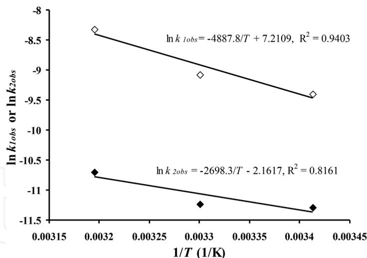
**Figure 6.** The Arrhenius plots of the intrinsic reaction rate constants at different temperature (in Kelvin) for PAA formation (molar ratio of acetic acid to  $H_2O_2 = 1:1$ , catalyst loading =  $471 \text{ mg/cm}^3$ ).
