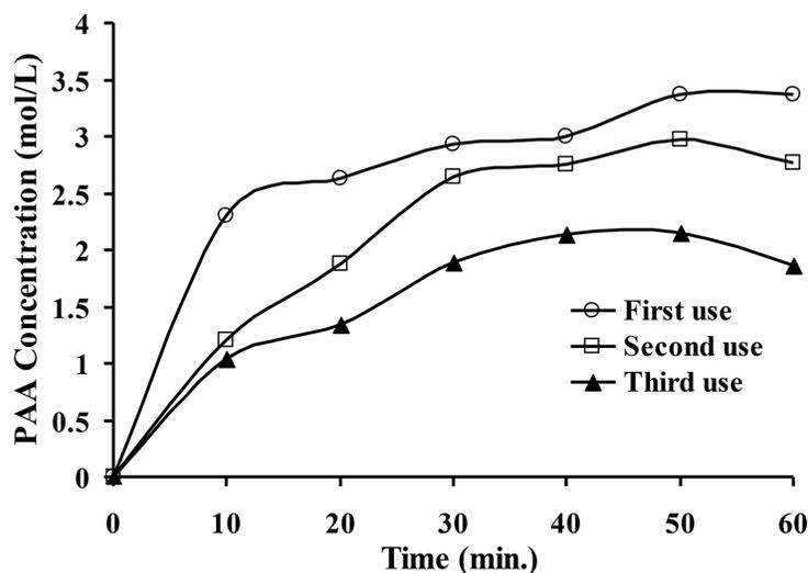
**Figure 7.** Deactivation of Amberlite IR-120H catalyst during PAA formation (molar ratio of acetic acid to  $H_2O_2 = 1:1$ , catalyst loading =  $471 \text{ mg/cm}^3$ , temperature =  $40^\circ\text{C}$ ).
