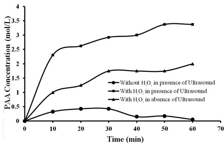
**Figure 9.** PAA formation in the presence of ultrasound without H<sub>2</sub>O<sub>2</sub>, in presence of ultrasound with H<sub>2</sub>O<sub>2</sub> and in the absence of ultrasound with H<sub>2</sub>O<sub>2</sub> (molar ratio of acetic acid to H<sub>2</sub>O<sub>2</sub> = 1:1, catalyst loading = 471 mg/cm<sup>3</sup>, and temperature = 40°C).
