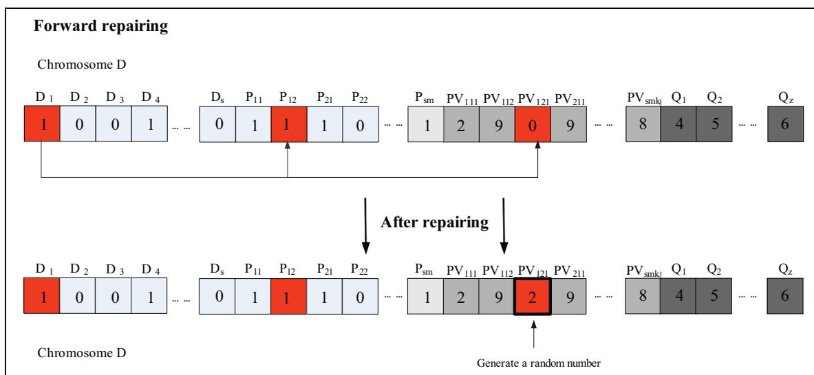
Fig. 4(a). Sample chromosome of forward repairing
