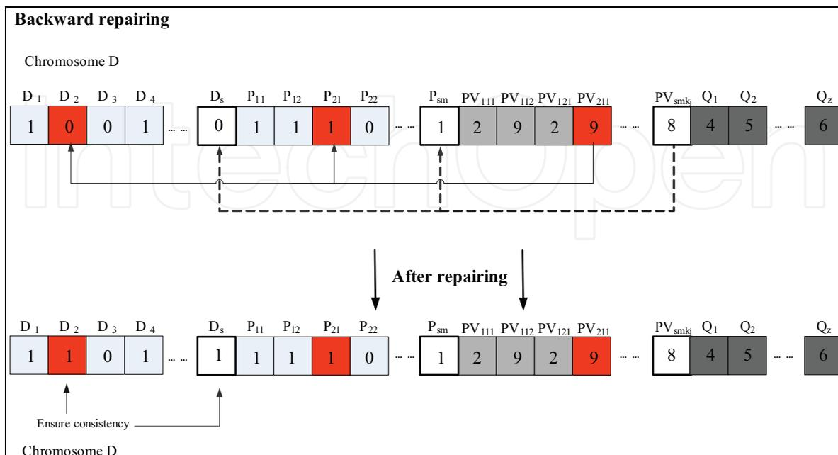
Fig. 4(b). Sample chromosome of backward repairing
