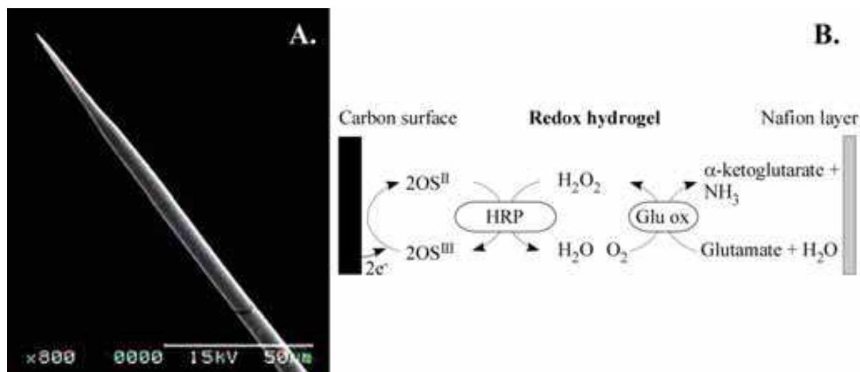
Fig. 9. (A) Scanning electron micrograph of a CF glutamate microbiosensor. Note the 7  $\mu\text{m}$  carbon fiber ends in submicron tip and protrudes from the glass insulation by about 100  $\mu\text{m}$  (courtesy of Kation Scientific). (B) Schematic of electrochemical detection of glutamate using osmium and oxidase-peroxidase enzymes containing redox hydrogel. Abbreviations: HRP, horse-radix peroxidase; Glu-ox, glutamate oxidase; OS, osmium.
