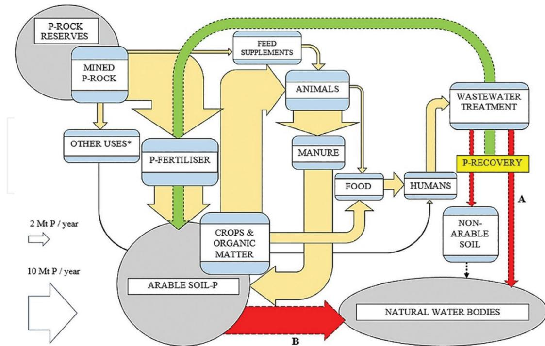
**Figure 1.** Diagram of key global P flows (the widths of the arrows semiquantitatively represents figures reported by Cordell [1] in million tons (Mt) of P per year. Point “A” denotes the flow of P contained in treated or untreated sewage to natural water bodies and represents approximately 1.5 Mt P/year. Point “B” denotes the flow of P contained in erosion losses and is about 8 Mt P/year. \*Other uses include industrial uses such as the production of some detergents) [9].
