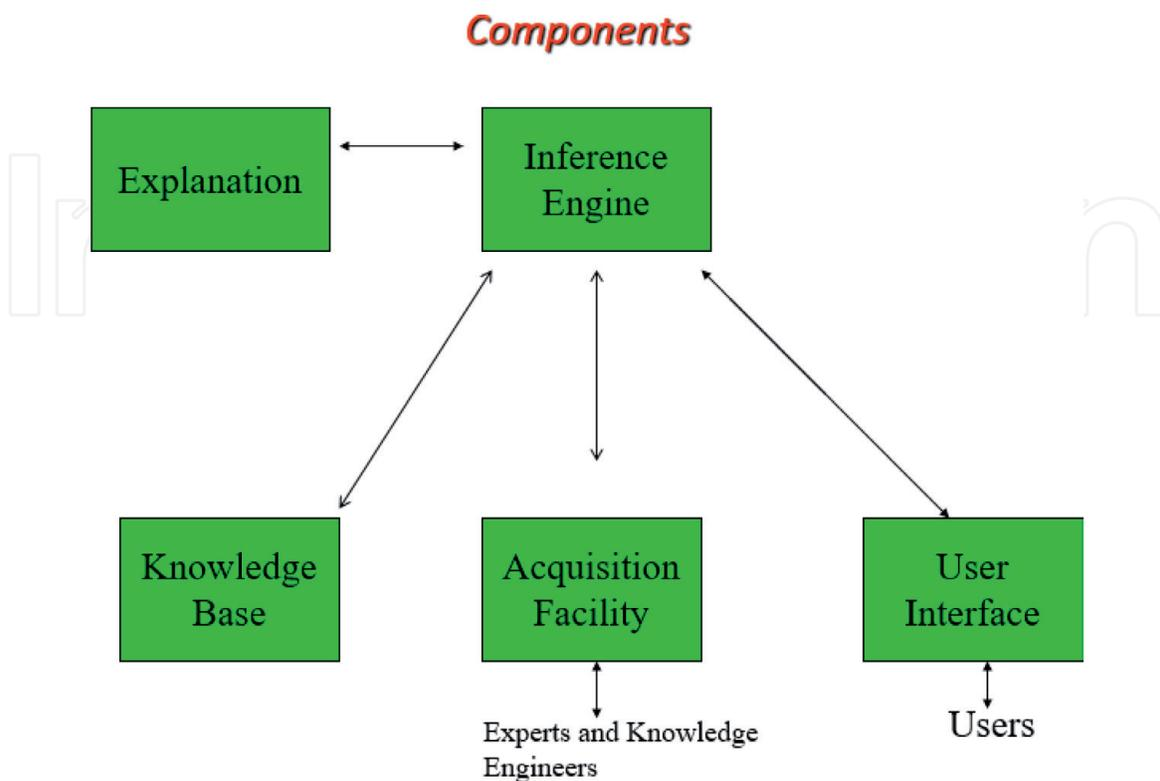
Figure 2. Main elements of an expert system.
