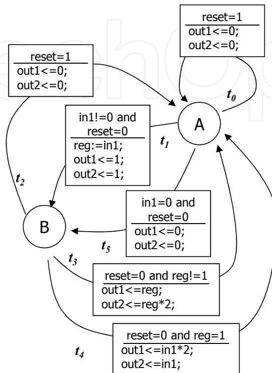
Fig. 2. State transition graph of an EFSM.
