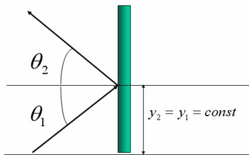
Fig. 8. Reflection from a planar mirror
