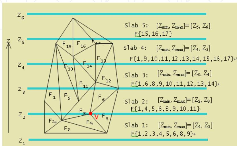
Fig. 12. The bucket-sorting algorithm for data sorting
