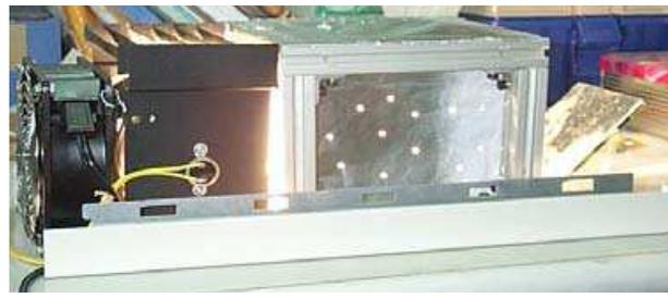
Fig. 5(a). The design of the curing light source; 5(b) Real structure of the curing light source
