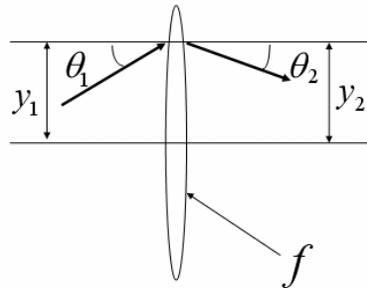
Fig. 7. Transmission through a thin lens
