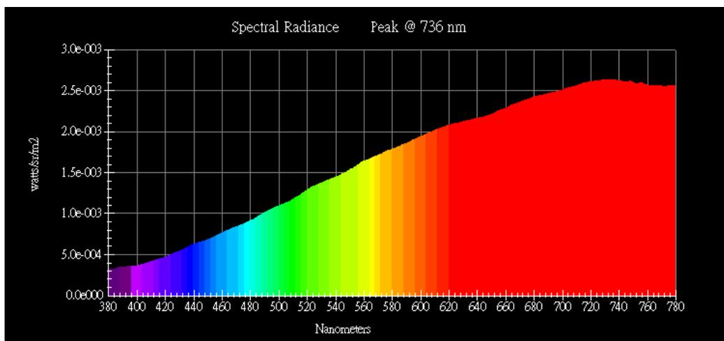
Fig. 4. The spectrogram of the 275W xenon lamp.
