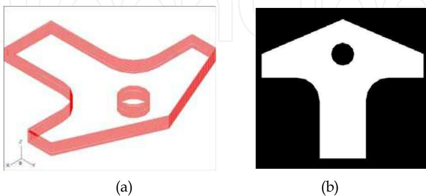
Fig. 19(a) Illustration of sliced model; Fig. 19(b) Cross contour displayed in the LCD photomask
