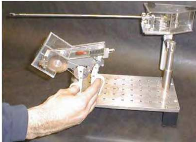
Figure 4. Force controlled gripper designed at the University of Washington (Rosen et al., 1999a)
