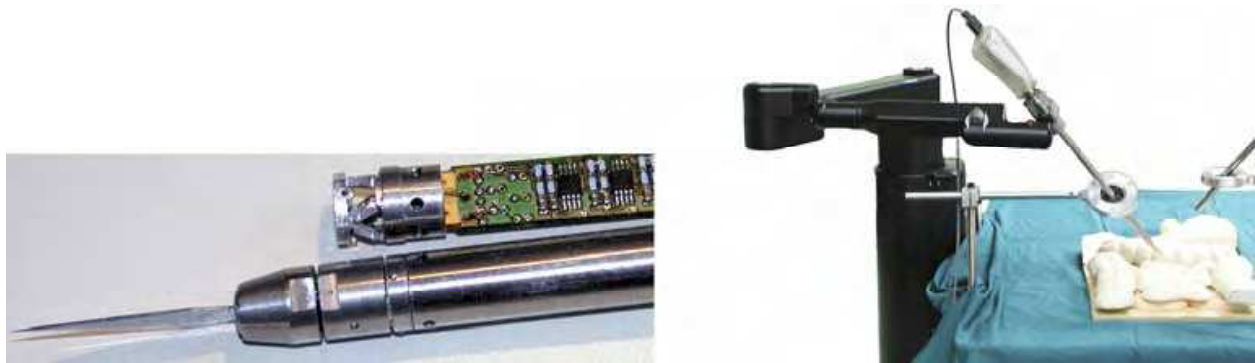
Figure 10. Application of the sensor in an experimental surgical knife, attached to a Zeus manipulator
