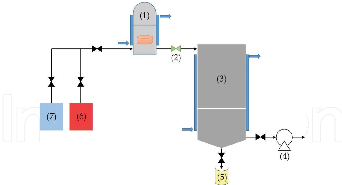
**Figure 2.** Schematic presentation of a typical DIC reactor: (1) treatment vessel, (2) controlled instant pressure drop valve, (3) vacuum tank with cooling jacket, (4) vacuum pump, (5) extract collection trap, (6) steam generator, and (7) air compressor.
