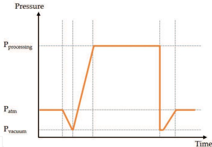
**Figure 3.** Pressure profile of a typical DIC treatment.
