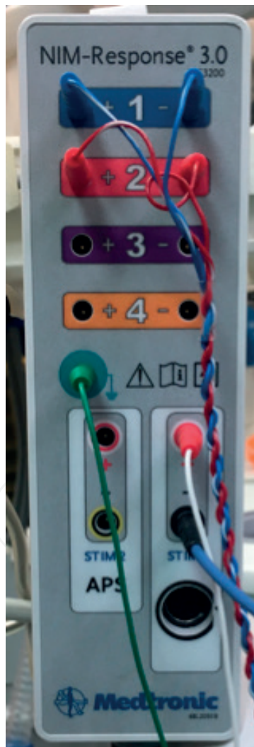
Figure 3. Stimulation and recording sides are combined on the interconnect box, through which they connect to the monitor.
