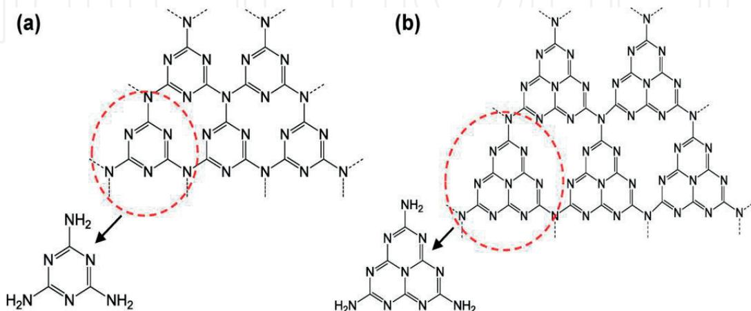
**Figure 1.** The basic tectonic units for g-C<sub>3</sub>N<sub>4</sub> photocatalyst (a) triazine and (b) tri-s-triazine (heptazine) structures. (Adapted with permission from Ref. [22]).
