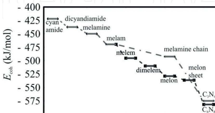
**Figure 3.** Calculated energy diagram for the development of C<sub>3</sub>N<sub>4</sub> using cyanamide as the precursor. Cyanamide was condensed to melamine. Further condensation proceeded by a triazine route (dash-dot line) or tri-s-triazine (dashed line). (Adapted with permission from Ref. [33]).
