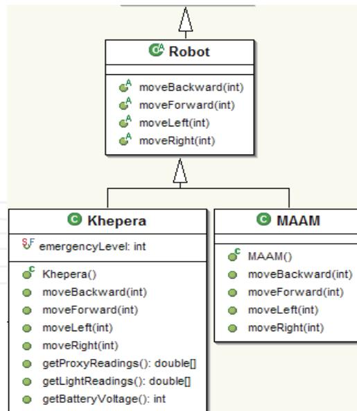
Fig. 2. UML class diagram of the robot primitives
