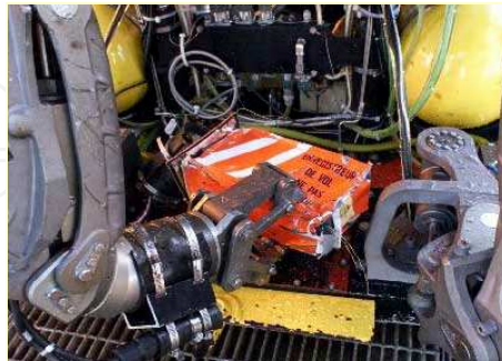
Fig. 4. black-box recovery using ROV, from U.S. Dept. of Defence.
