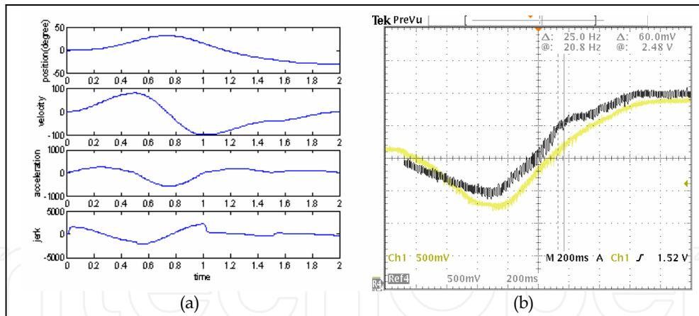
Figure 14. The initial position of an actuator is zero. Three goal positions are commanded at times 0, 1, and 1.5 seconds respectively:  $p_T(0) = 40$ ,  $p_T(1) = 10$ ,  $p_T(1.5) = -30$ . The velocity function can be obtained by merging the three bell-shaped velocity profiles, which are created at 0, 1, and 1.5 seconds, respectively: (a) simulation results and (b) experimental results
