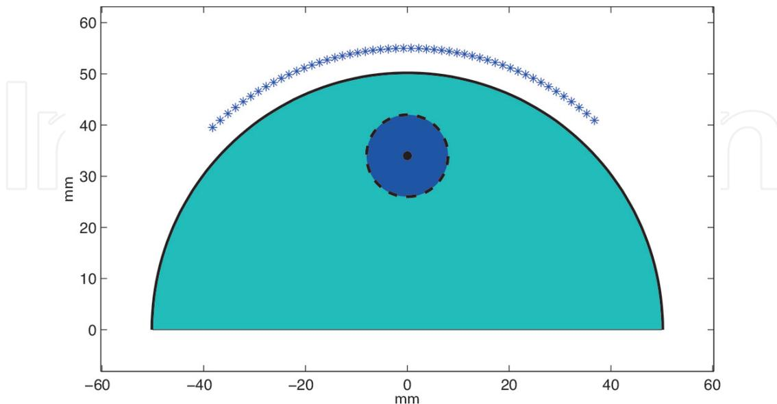
**Figure 1.** A schematic 2-D breast model with a 16-mm embedded tumor at  $(0, 34)$  as a reference geometry. A curvilinear ultrasonic array with 51 transducers is located near to the organ at risk. The ultrasonic array is used for hyperthermia treatment.
