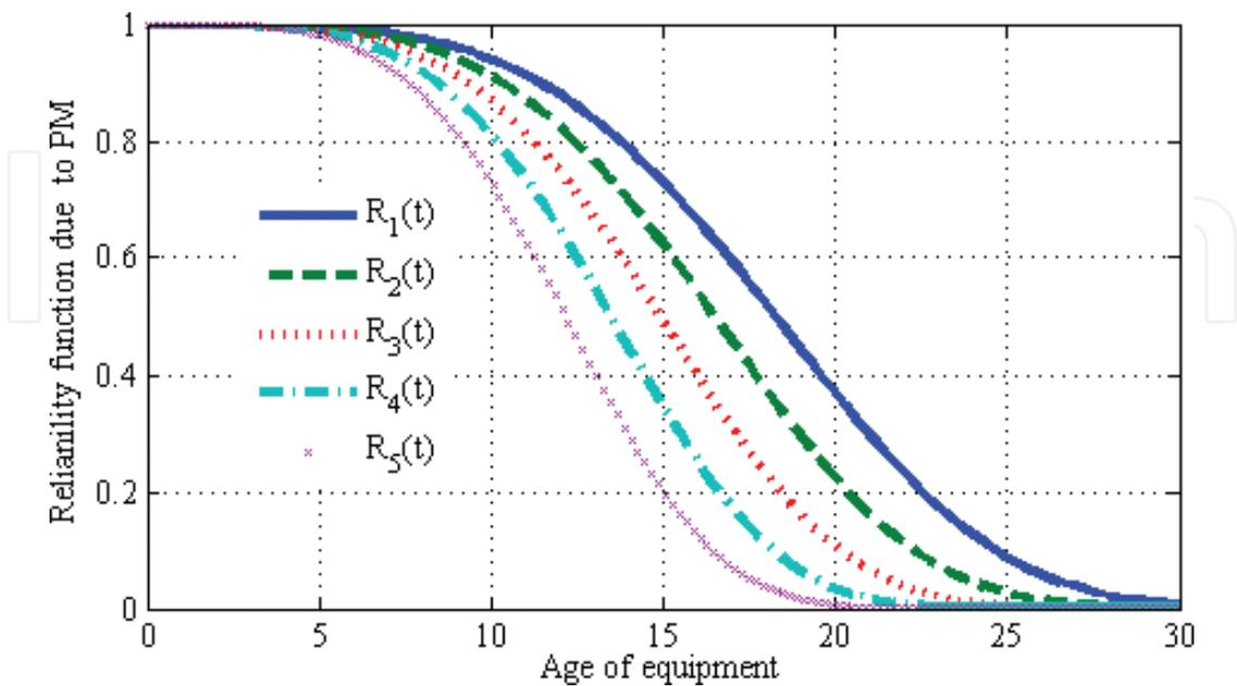
Figure 2. Evolution of reliability function due to preventive maintenance.
