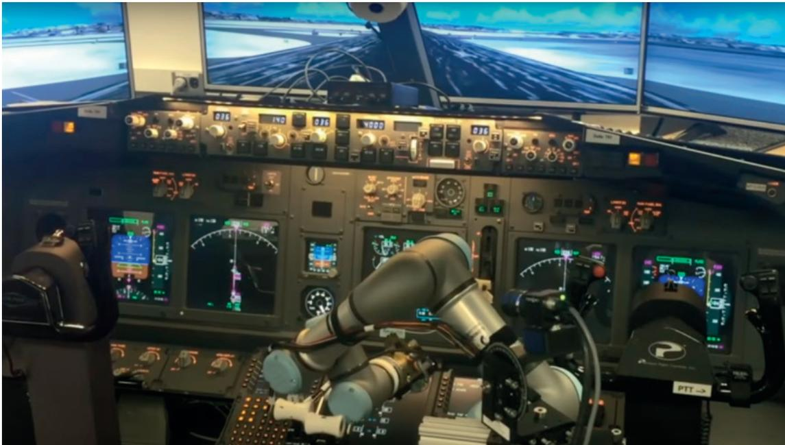
Figure 1. Robotic co-pilot ALIAS landing a Boeing 737.
