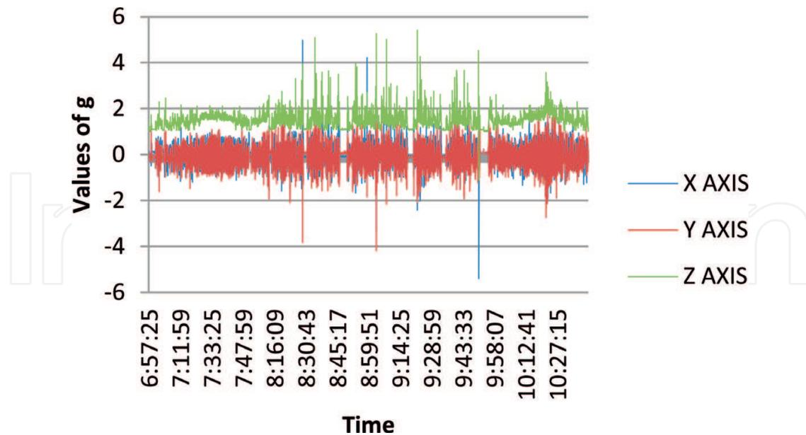
Figure 3. Values of acceleration coefficients (Brno–Vyškov and return).
