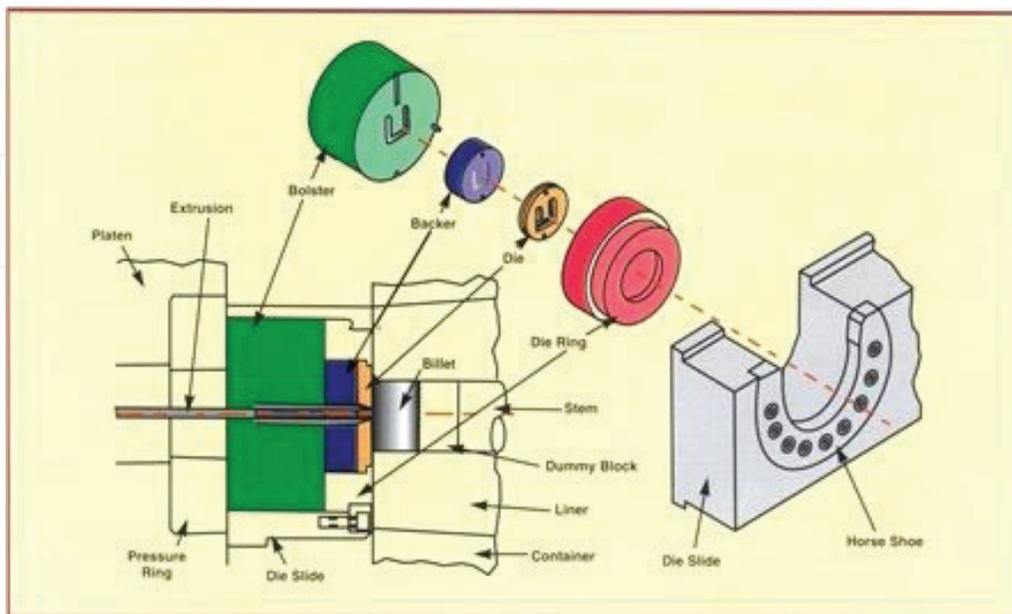
**Figure 1.** Major components of the metal extrusion press.
