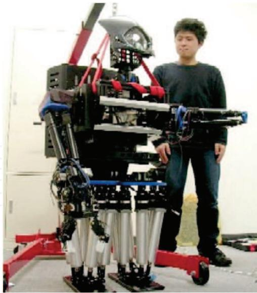
Fig. 3. Rescue robot partly powered by the laser
