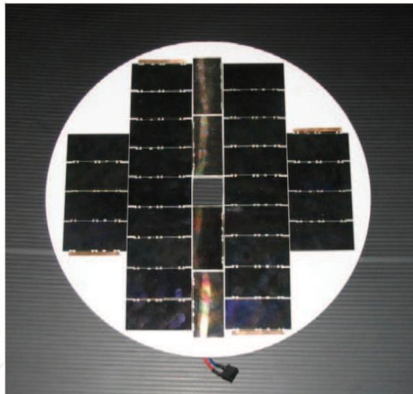
Fig. 5. Solar panel for a kite plane drive
