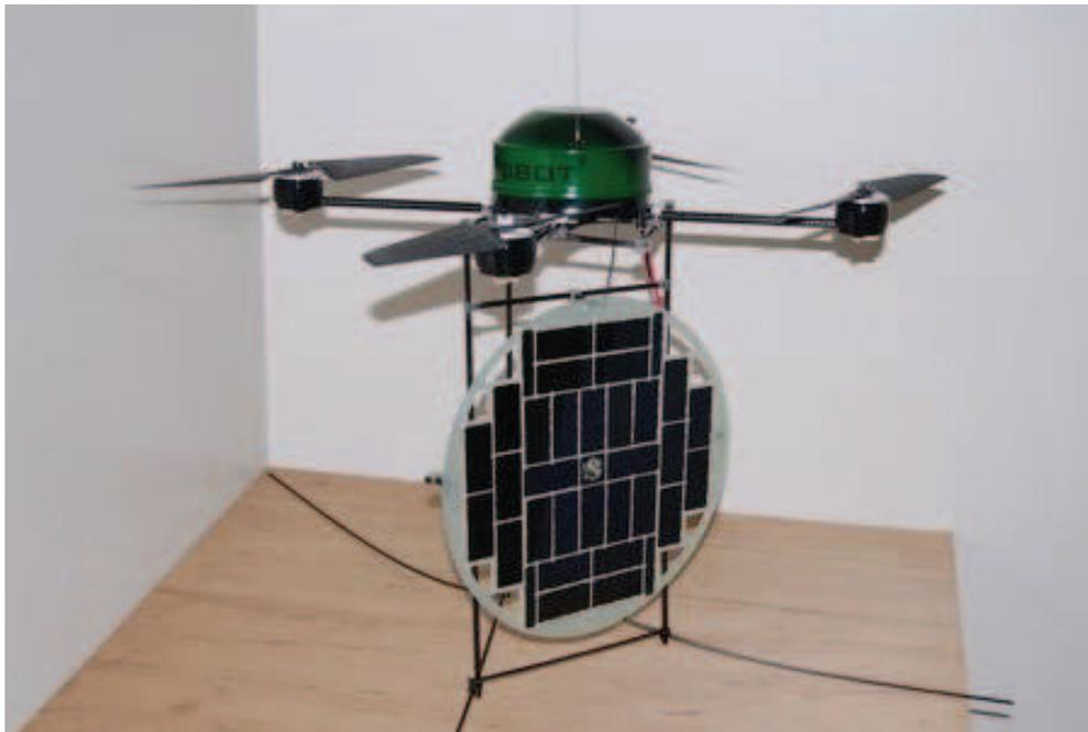
Fig. 8. Helicopter with a vertical solar panel underneath
