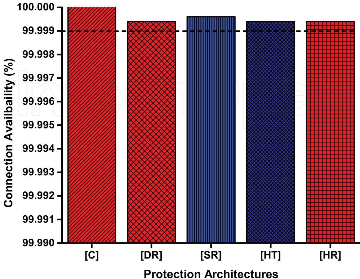
Figure 8. Overall connection availability of selected protection architectures.
