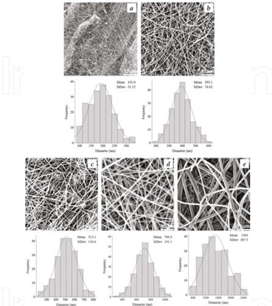
**Figure 5.** SEM micrographs and diameter distribution of electrospun fibres produced by needleless electrospinning with silk fibroin solution at various concentrations : (a) 6 wt%; (b) 8 wt%; (c) 10 wt%; (d) 12 wt%; (e) 14 wt% (magnification 5 $\times$ ).
