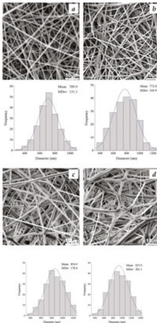
**Figure 4.** SEM micrographs and diameter distribution of electrospun fibres prepared from silk fibroin 12 wt% with varying amounts of  $\text{CaCl}_2$ : (a) 1:0.25; (b) 1:0.30; (c) 1:0.35; (d) 1:0.40; (SEM magnification 5 $\times$ ).
