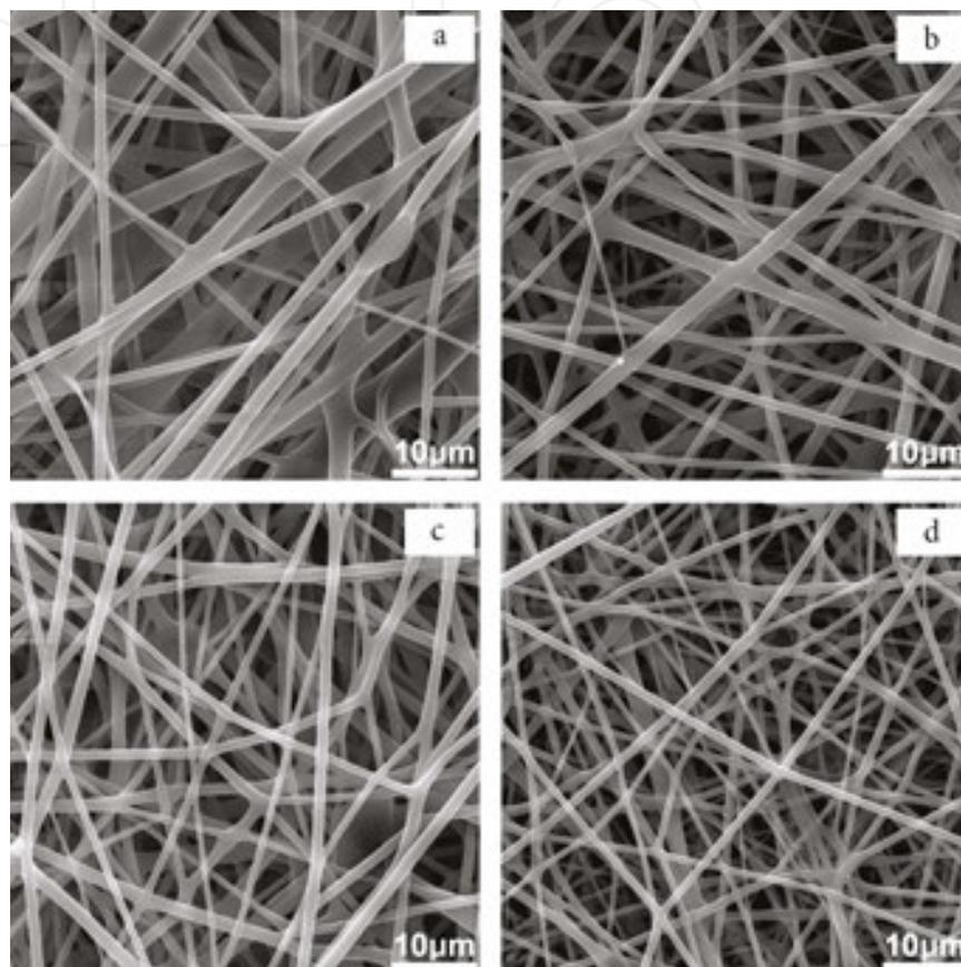
**Figure 7.** SEM micrographs and diameter distribution of electrospun fibres prepared by needleless electrospinning from silk fibroin 12 wt% at various applied voltages: (a) 30 kV; (b) 40 kV; (c) 50 kV; (d) 60 kV (SEM magnification 5 $\times$ ).
