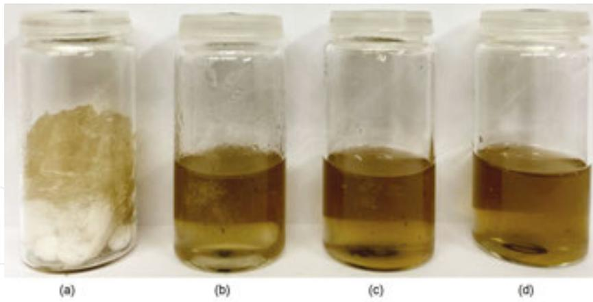
**Figure 3.** The dissolution of silk fibroin in formic acid with varying amounts of calcium chloride: (a) without  $\text{CaCl}_2$ ; (b) 1:0.15; (c) 1:0.20; (d) 1:0.25 [SF:CaCl<sub>2</sub> (w/w)].
