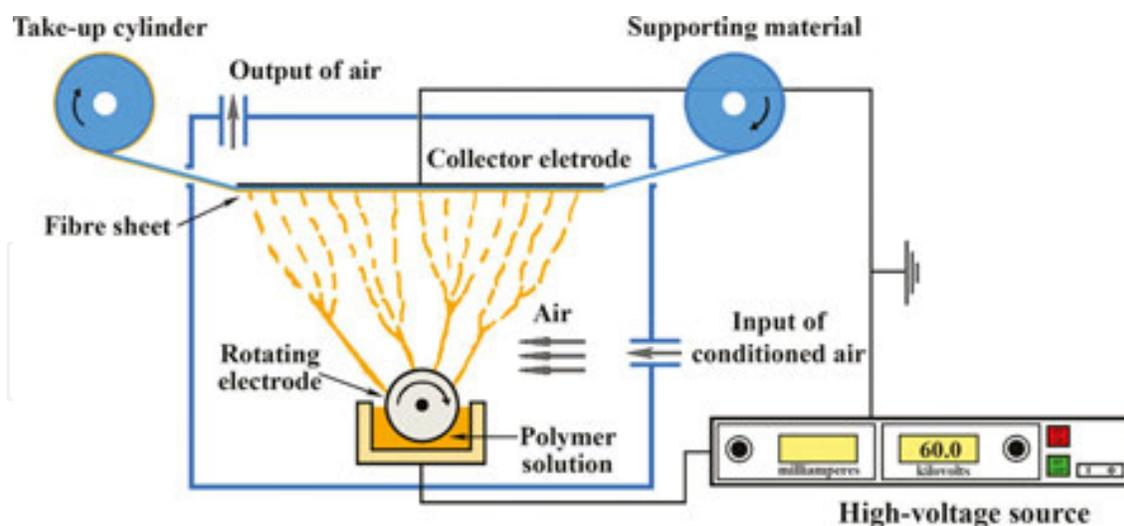
Figure 1. Schematics of the needleless electrospinning setup.
