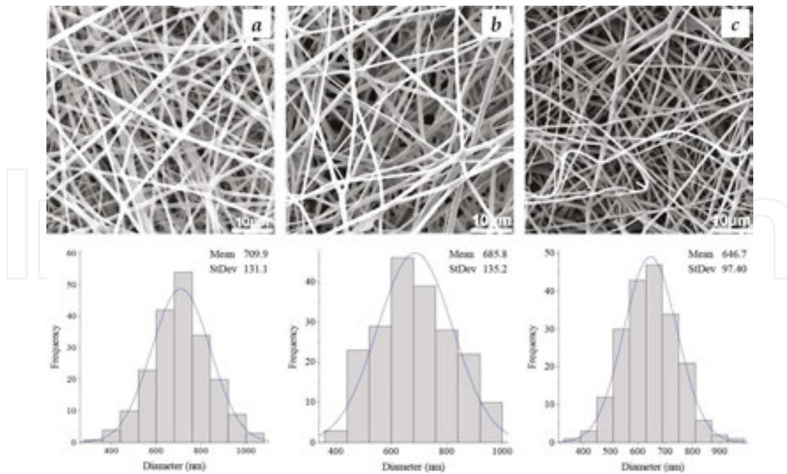
**Figure 9.** SEM micrographs and diameter distribution of electrospun fibres prepared by needleless electrospinning from silk fibroin 12 wt% at different spinning distance: (a) 100 mm; (b) 125 mm; (c) 150 mm (SEM magnification 5 $\times$ ).
