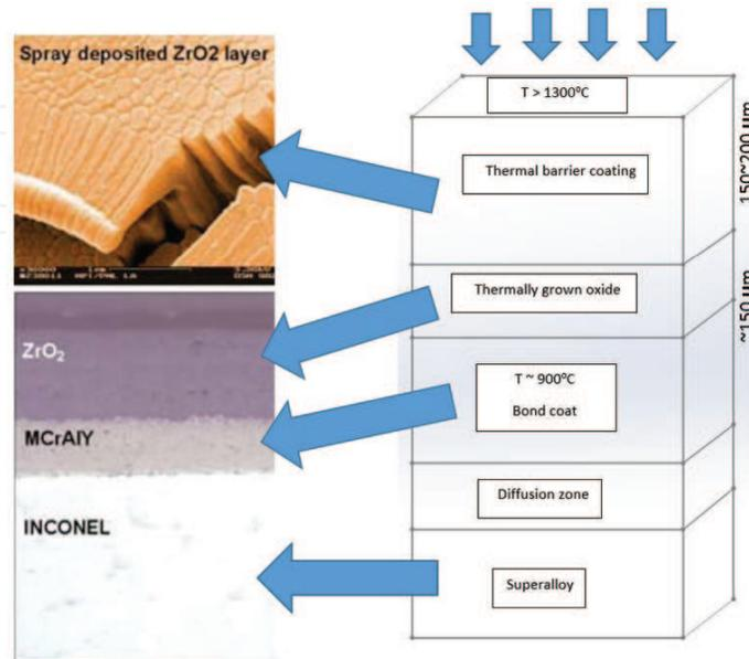
**Figure 7.** Schematic view of TBC coating system.
