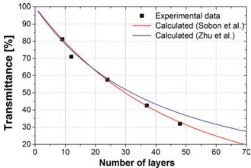
**Figure 11.** Optical transmittance of multilayer graphene: calculated from formula (1) (red line, no interaction between layers), calculated from formula (2) (blue line, including layer interactions), and measured using multilayer graphene (dotted line) [67].
