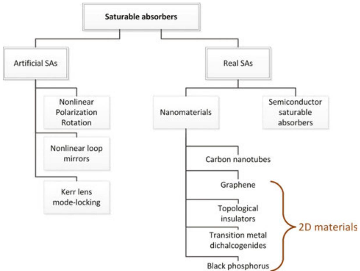
**Figure 3.** Types of saturable absorbers for ultrafast lasers.
