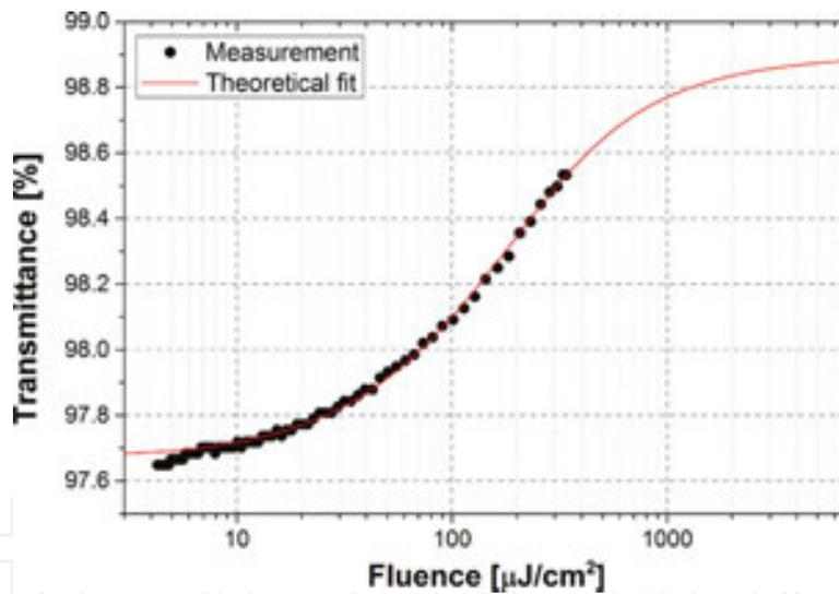
**Figure 9.** Measurement of saturable absorption in monolayer graphene.
