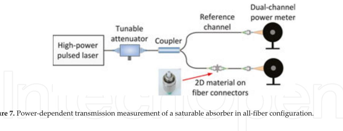
**Figure 7.** Power-dependent transmission measurement of a saturable absorber in all-fiber configuration.
