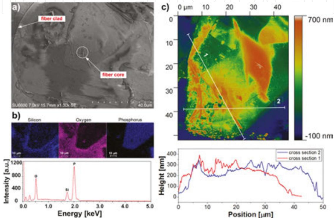
**Figure 14.** Characterization of the mechanically exfoliated BP layers transferred onto an optical fiber: (a) SEM image with marked fiber clad and core, (b) EDX spectroscopy data, (c) AFM image of the core area, and (d) cross section through the fiber core area indicating approx. 200–300 nm height of the BP flake on the core.
