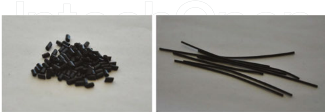
Figure 9. Graphene infused PLA pellets and 1.75 mm filaments.
