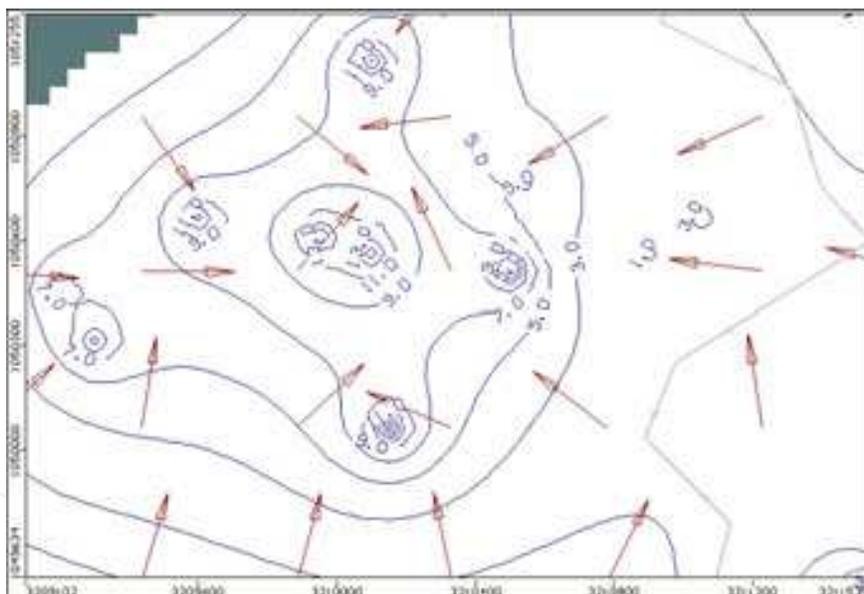
Figure 14c. Cone of depression in layer 7 (1-year simulation in 2008, non-steady state).
