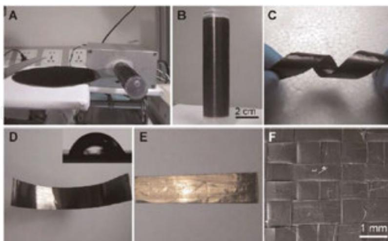
**Figure 2.** Pure CNT assembly films can be produced by layer-by-layer stacking of as-drawn CNT sheets with the aid of solvent densification [87] (A) Setup for layer-by-layer stacking of aligned CNT sheets. (B) As-prepared CNT film on a mandrel. (C) Flexible CNT film strip. (D,E) Photographs of a shining CNT strip and a strip coated with a 12 nm gold layer. Inset in (D) is the shape of a water droplet on the strip. (F) SEM image of a woven fabric consisting of CNT strips.
