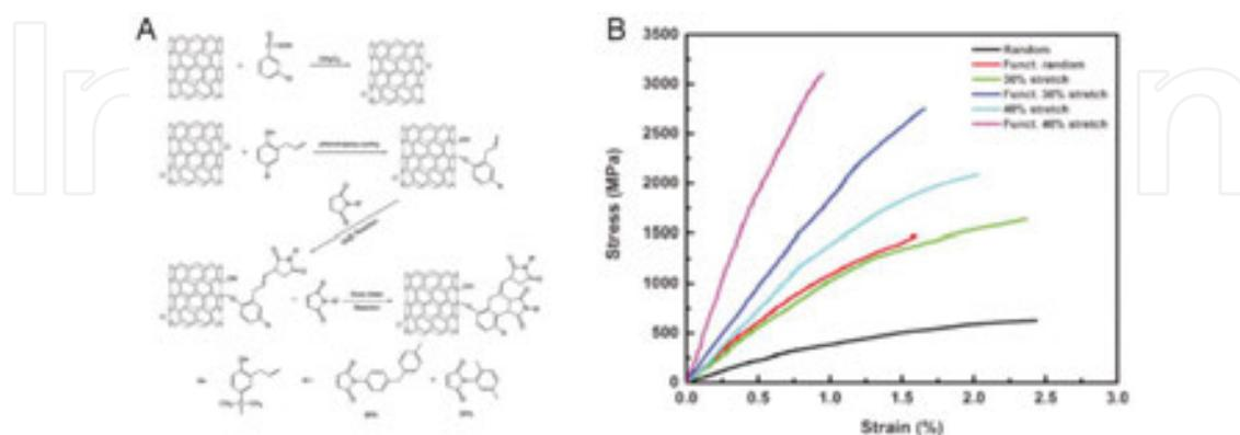
**Figure 5.** CNT functionalization improved the interfacial bonding strength and thus increased the tensile properties of the CNT/BMI composites [95]. (A) Proposed reaction mechanism of functionalized CNTs and BMI resin. (B) Typical tensile stress–strain curves of random and stretch-aligned CNT/BMI composites with and without functionalization.
