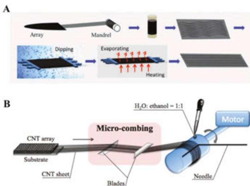
**Figure 3.** Two solutions to further improve the CNT alignment. (A) CNT alignment can be remarkably improved by the stretch-dip-drying method [88]. (B) Schematic view of the microcombing process which can mitigate the CNT waviness [89].
