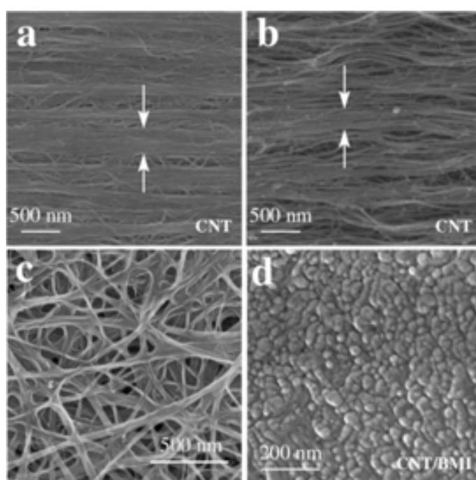
**Figure 7.** SEM characterization of different CNT assembly structures [24]. (A) CNT aggregation in the layer-by-layer stacking of as-spun aligned CNT sheets. (B) CNT aggregation in the stretched dry films composed by entangled CNTs. (C) Acetone-densified CNT webs maintained the feature of entanglement. (D) Cross section of the optimal CNT/BMI composite structure using focused ion beam treatment, where the aggregation level of CNTs was limited within a dimension of 20–50 nm.
