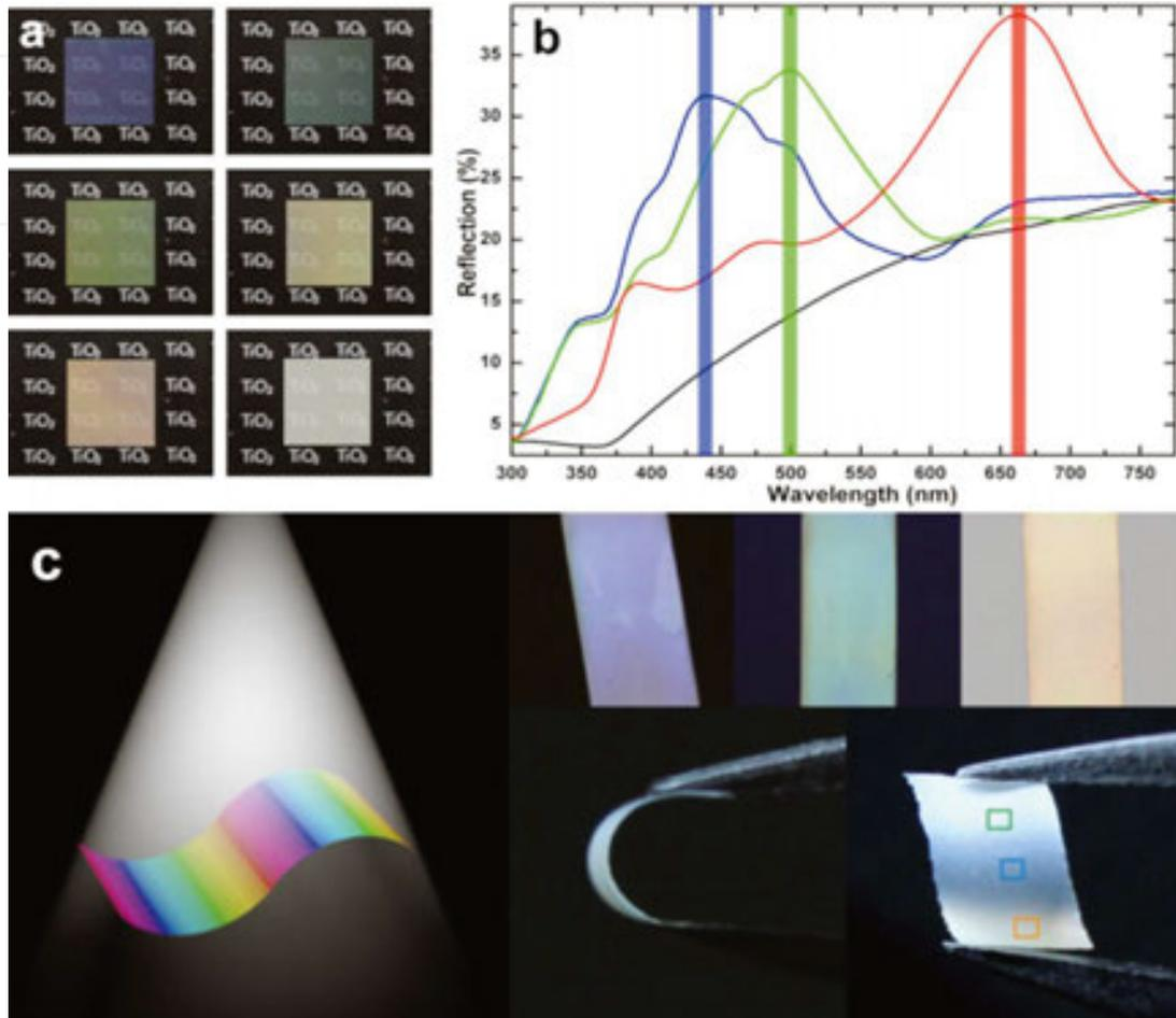
**Figure 8.** The optical images of the colorful films, from purple to red. (b) The reflection spectra of the colorful films, showing the bandgaps. (c) The change of film colors with different incident and viewing angles and the flexibility of the colorful films. Reprinted with permission from Lin et al. [45].
