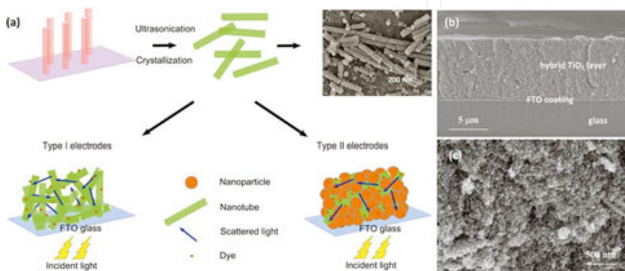
**Figure 4.** The schematic of the fabrication procedures of nanotube powders, nanotube electrode, and hybrid electrode. (b, c) The cross-sectional views of the hybrid photoanode with nanotubes embedded in nanoparticles. Reprinted with permission from Lin et al. [27].
