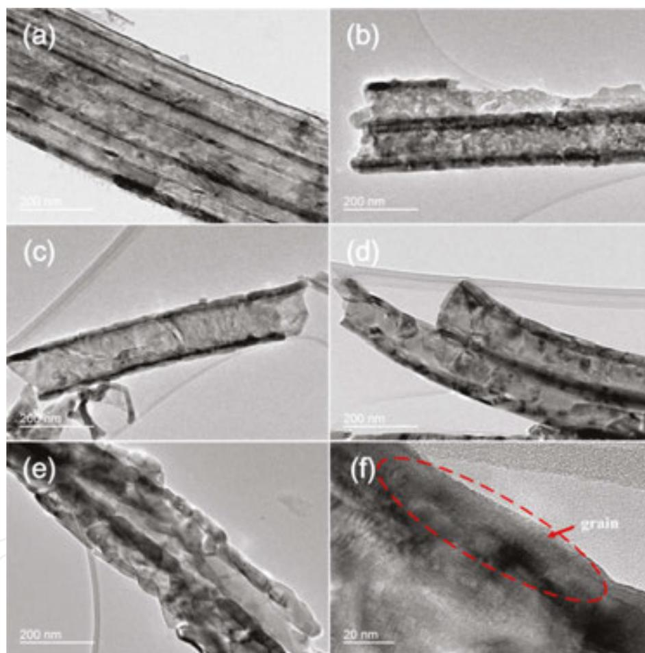
**Figure 9.** TEM images of tube membranes annealed at (a) 400, (b) 500, (c) 600, (d) 700, and (e)  $800^\circ\text{C}$ . (f) HRTEM view of the grain in the tube walls annealed at  $700^\circ\text{C}$ . Reprinted with permission from Lin et al. [59].
