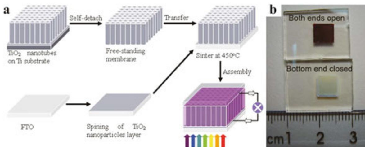
**Figure 2.** (a) Scheme of the fabrication procedure of front-side illuminated DSSCs using detached nanotube layers. (b) The photographs of the oxide layers with open and closed bottoms adhered onto FTO substrates. Reprinted with permission from Lin et al. [20].
