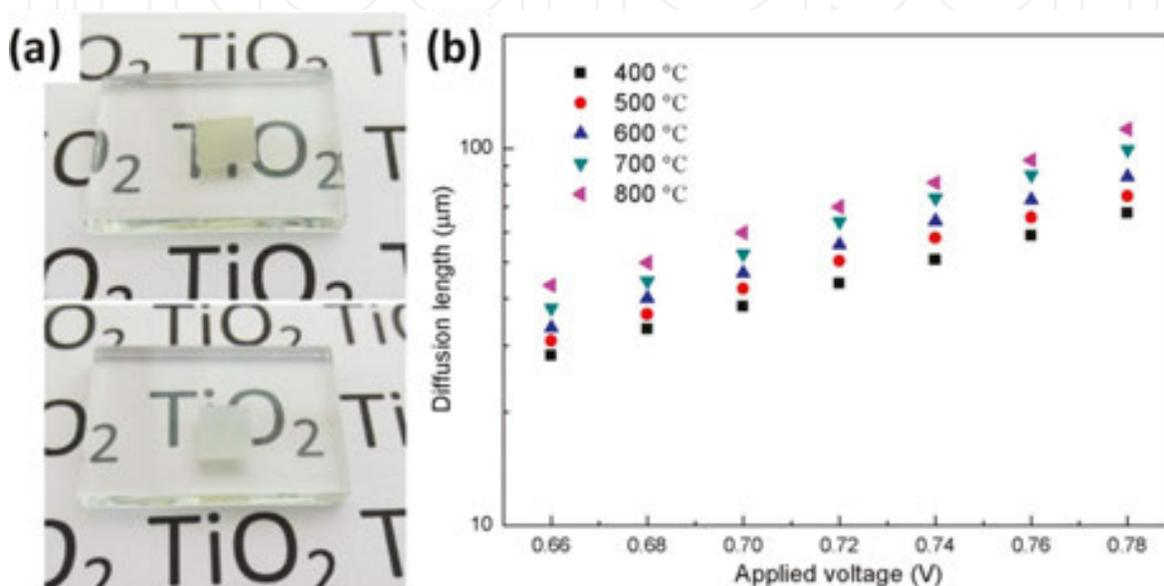
**Figure 10.** (a) The photographs of photoanodes consisting nanotube membranes annealed at 400 and 700°C. (b) The variation of diffusion length in DSSCs as a function of annealing temperature. Reprinted with permission from Lin et al. [59].
