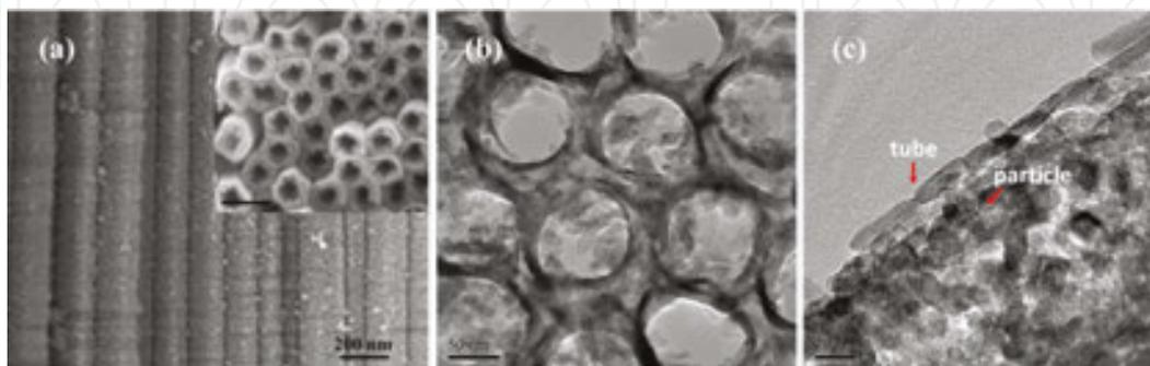
**Figure 11.** (a) The cross-sectional SEM images of the hybrid tubes by water immersion treatment. The insert is the top view. (b, c) TEM images of the hybrid structure consisting tubes and particles. Reprinted with permission from Lin et al. [63].
