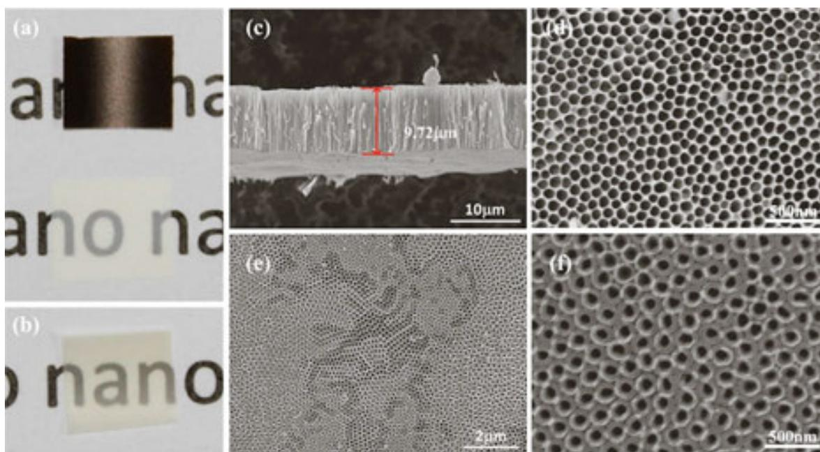
**Figure 1.** The photographs of (a) the detached 200°C-treated oxide layer with open bottoms before and after annealing and (b) the detached 400°C-treated oxide layer with closed bottoms. SEM images of the detached 200°C-treated oxide layer with (c) the cross-sectional view, (d) the top view, (e) the bottom view showing the open morphology, and (f) the enlarged bottom view. Reprinted with permission from Lin et al. [17].
