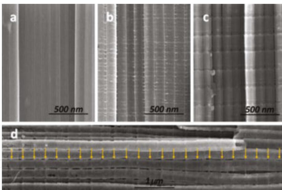
**Figure 7.** The cross-sectional SEM image of the periodic structures with (a) smooth, (b) rippled, and (c) periodic tubes with concave interfacial morphologies. (d) The periodic structures along the tube axis with long-range regularity (period length: 292 nm). Reprinted with permission from Lin et al. [45].
