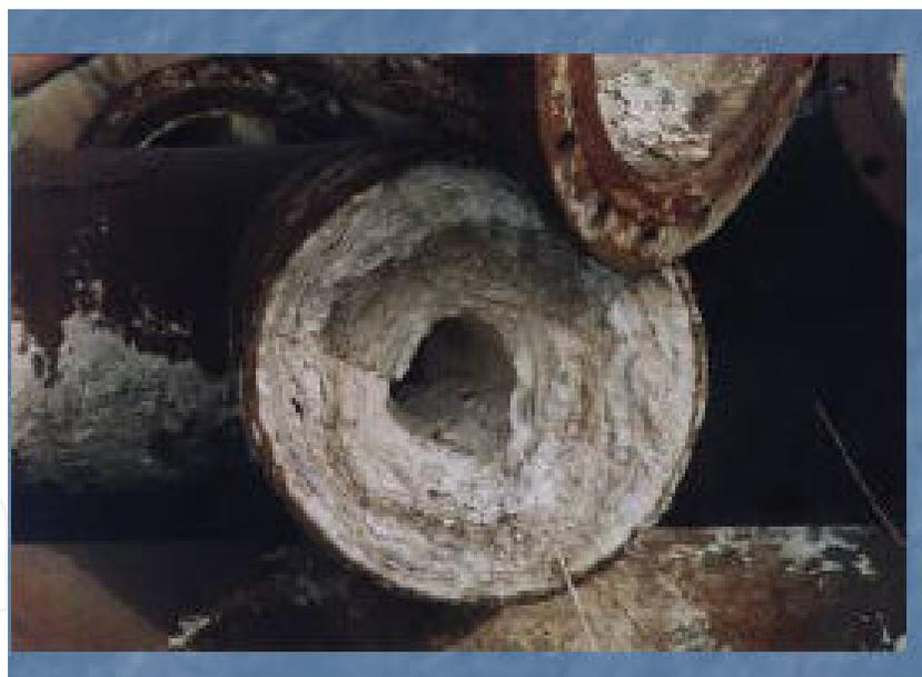
**Figure 4.** The build-up of scale on the interior of a pipe
