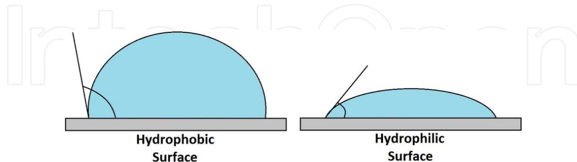
Figure 3. Principle of contact angle measurement
