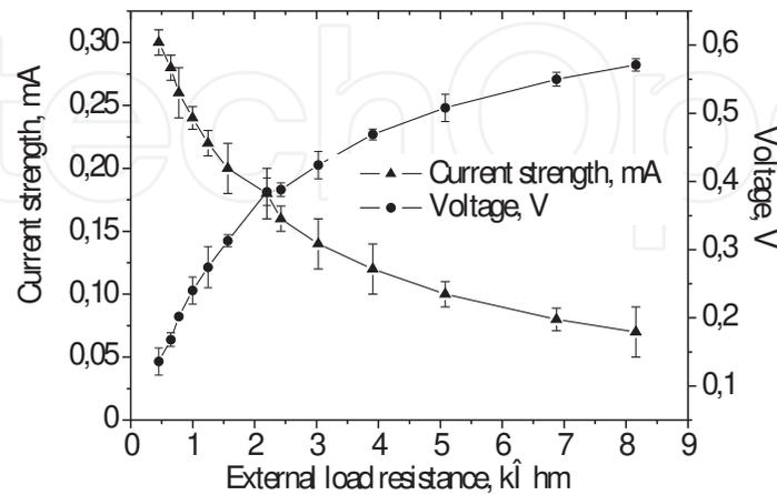
**Figure 8.** Volt-ampere characteristic of constructed MFC under the influence of various external load resistances on the third-beginning of the fourth days of *D. acetoxidans* IMV B-7384 growth under normal cultivation conditions
