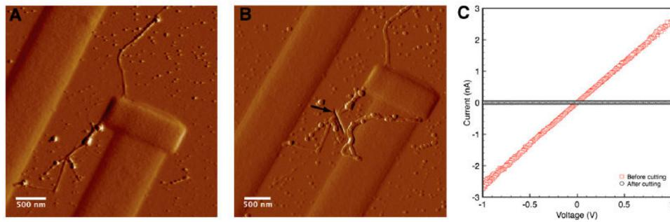
**Figure 1.** Measuring electrical transport along a bacterial nanowire. (A) Tapping-mode atomic force microscopy (AFM) amplitude image detailing the contact area with the bacterial nanowire from Fig. 1. (B) Contact-mode AFM deflection image of the junction after cutting the nanowire with FIB milling. The arrow marks the cut location. (C) Current-voltage curve of the bacterial nanowire (ramp-up and ramp-down) both before (red) and after (black) cutting the nanowire [52].
