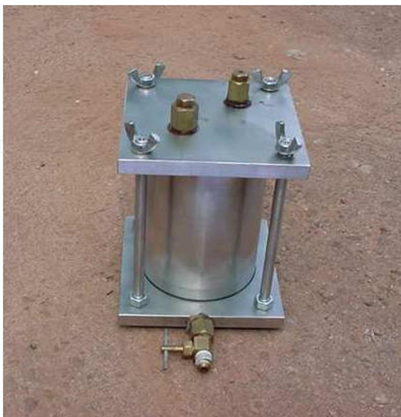
Figure 2. Hydraulic Conductivity cell.
